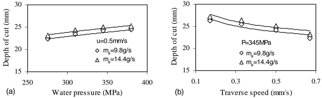
Fig. 1. Predicted and experimental depth of cut for straight cutting (standoff distance  $d=2\text{mm}$ ).
