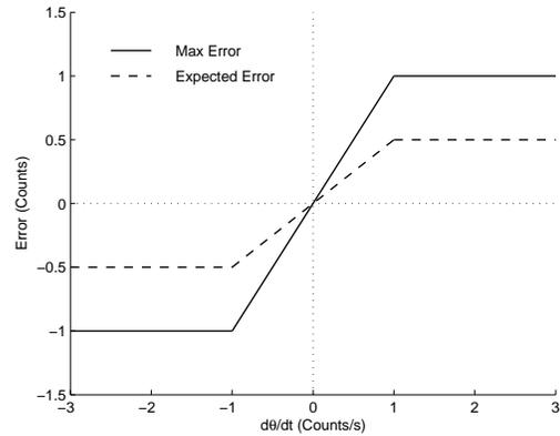
Fig. 2. Quantizing errors showing maximum and expected values
