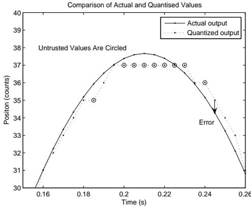
Fig. 1. Quantizing effects showing trusted and untrusted values
