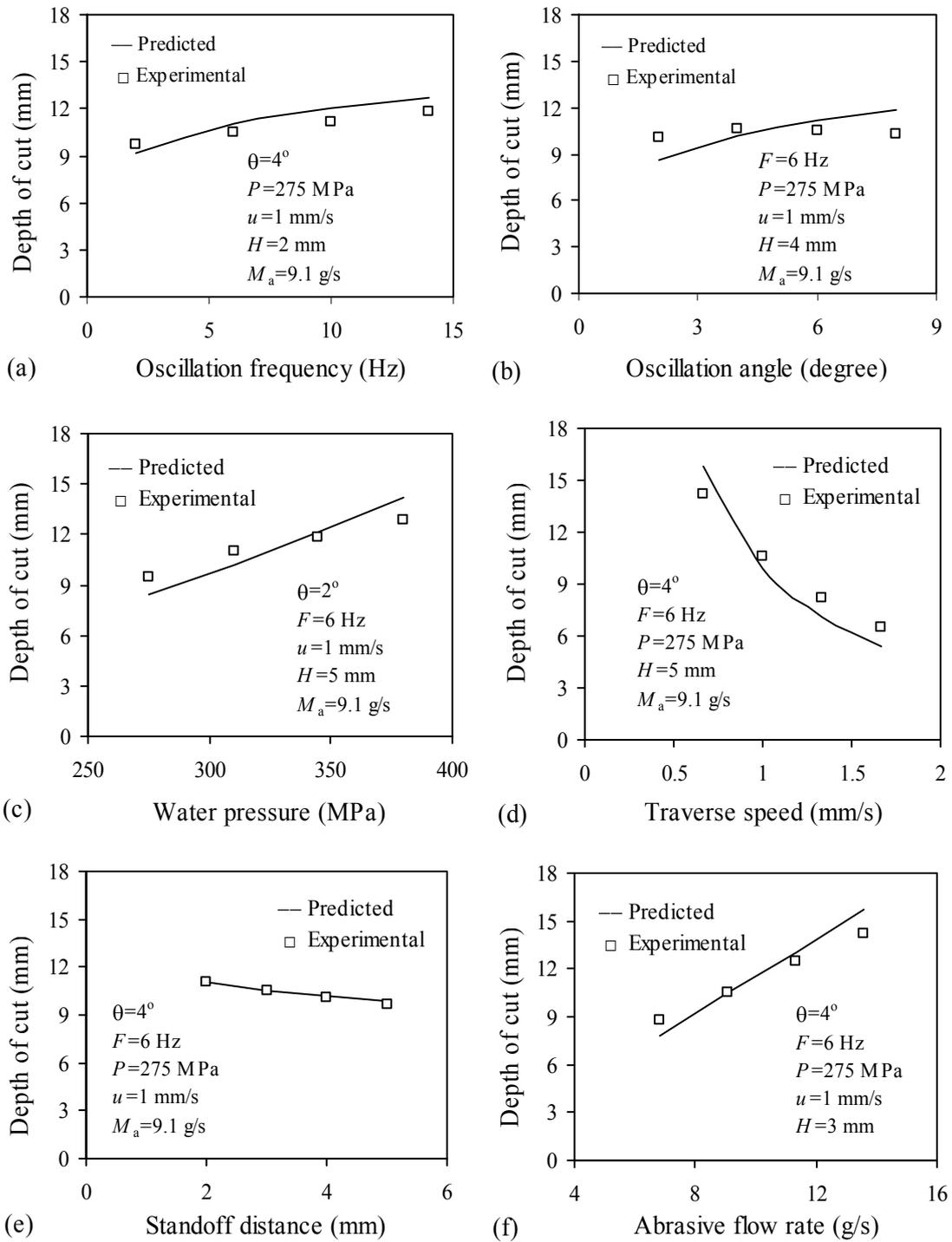
Fig. 5. Comparisons between model predictions and experimental data for nozzle oscillation cutting.
