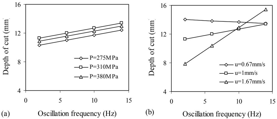
Fig. 2. Effect of oscillation frequency on the depth of cut: (a)  $\theta=4^\circ$ ,  $u=1\text{mm/s}$ ,  $H=2\text{mm}$ ,  $m_a=9.1\text{g/s}$ ; (b)  $\theta=4^\circ$ ,  $P=310\text{MPa}$ ,  $H=2\text{mm}$ ,  $m_a=9.1\text{g/s}$ .
