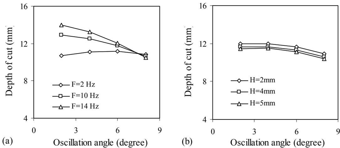
Fig. 3. Effect of oscillation angle on the depth of cut: (a)  $P=310\text{MPa}$ ,  $u=1\text{mm/s}$ ,  $H=3\text{mm}$ ,  $m_a=9.1\text{g/s}$ ; (b)  $F=6\text{Hz}$ ,  $P=310\text{MPa}$ ,  $u=1\text{mm/s}$ ,  $m_a=9.1\text{g/s}$ .
