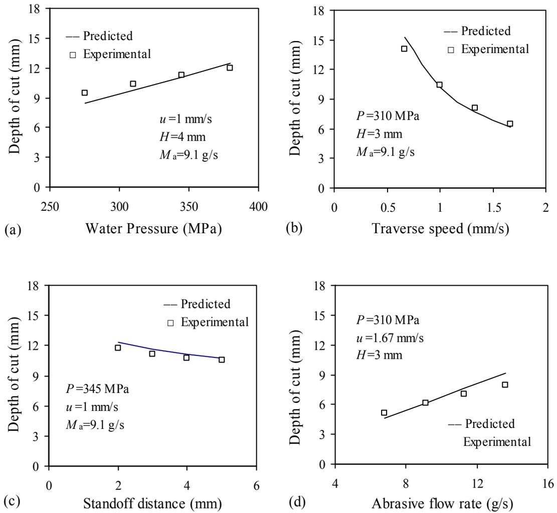
Fig. 4. Comparisons between model predictions and experimental data for cutting without nozzle oscillation.
