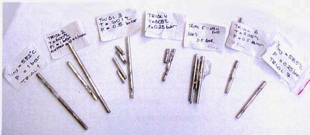
Figure 3.19: Injection die-cast amorphous \text{Mg}_{65}\text{Cu}_{25}\text{Y}_{10} samples generated using the tube die.
