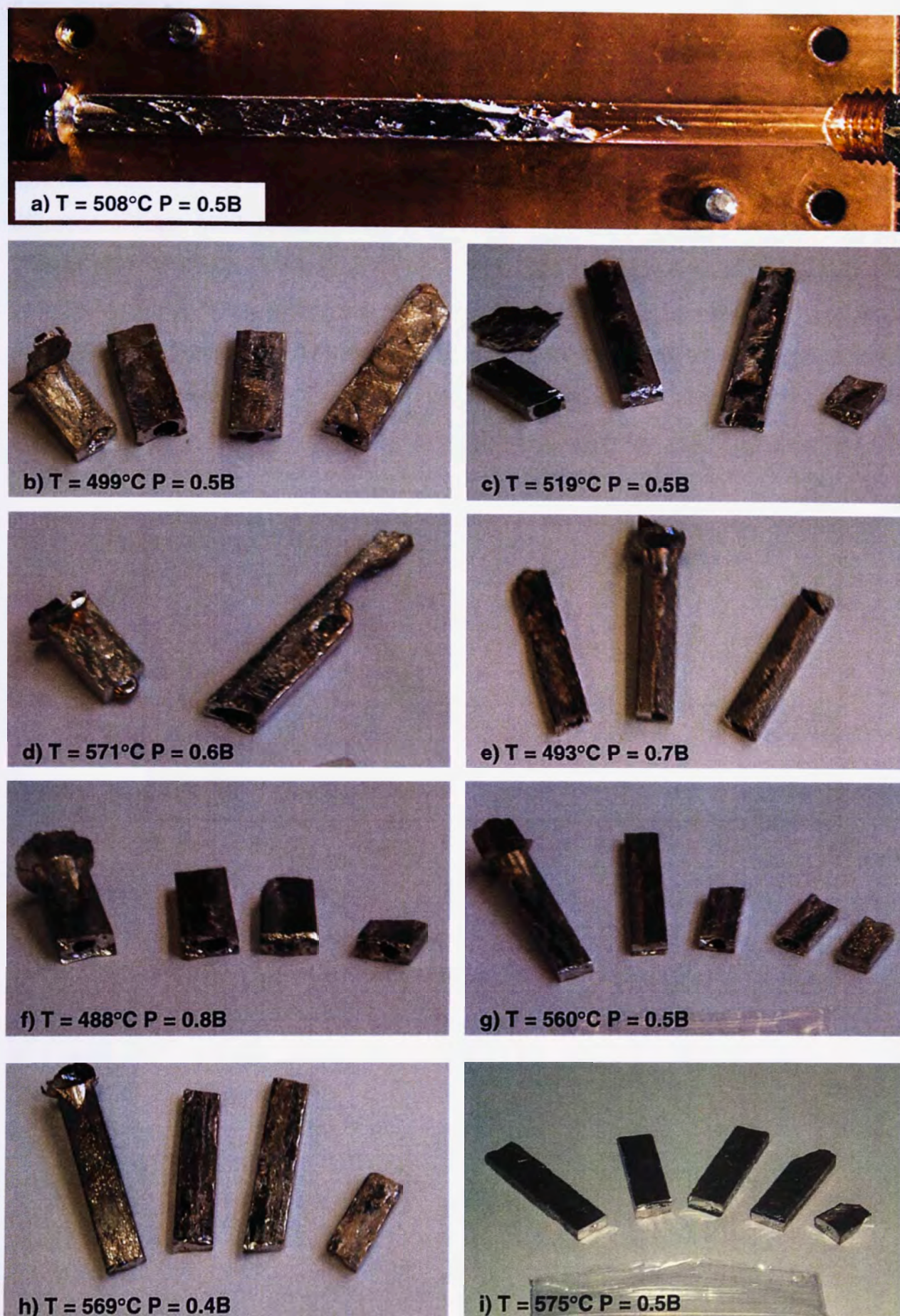
Figure 3.26: A range of amorphous \text{Mg}_{65}\text{Cu}_{25}\text{Y}_{10} samples produced by injection casting for a given combination of melt injection temperature and casting pressure.
