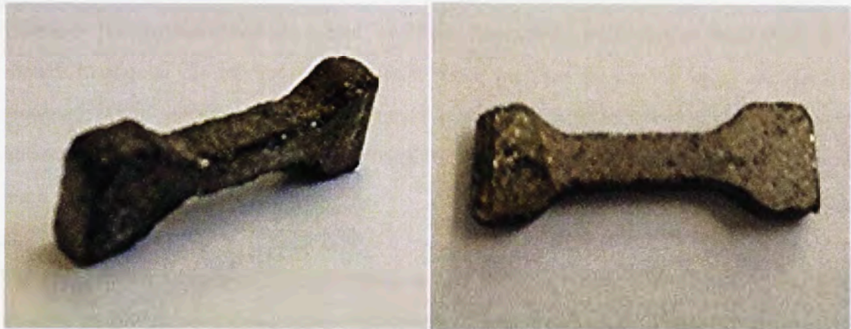
Figure 3.15: A tensile specimen of 3mm thickness produced by water jet cutting.
