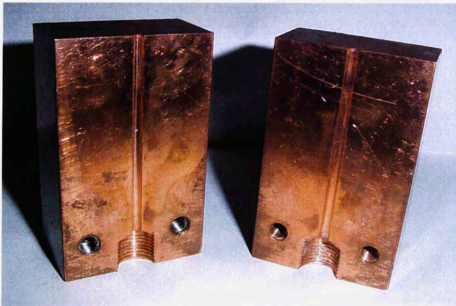
Figure 3.18: The tube or rod die. The die was originally twice the length given in this figure but was subsequently modified (cut in half) for aiding gas evacuation and for ensuring complete filling of the cavity.
