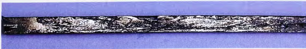
Figure 4.21: A sample cast at 450 °C and 1.5 Bar showing poor mould wall replication and the generation of cold shuts and porosity.
