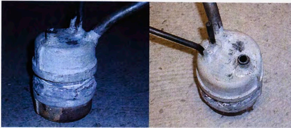
Figure 3.17: Prototype injection caster constructed out of cast iron irrigation fittings with appropriate plumbing fixtures.
