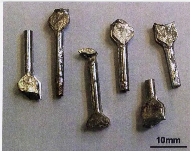
Figure 3.23: Unsuccessful injection-cast tensile test samples generated using the 'dog bone' die of Figure 3.22 .
