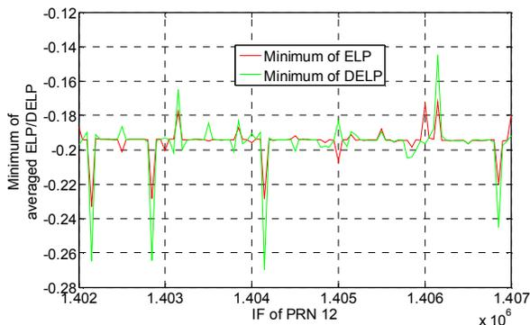
**Figure 10 – Comparison of minimum values of averaged ELP with that of DELP for PRN 12 in the presence of PRN 25 (IF=1405150 Hz) and multipath in PRN 12 signal with relative amplitude of 0.3 and phase difference of  $0.4918\pi$**
