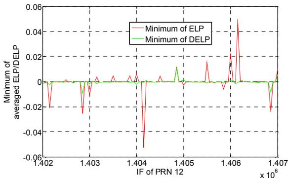
**Figure 14 – Comparison of minimum values of averaged ELP with that of DELP for PRN 12 in the presence of PRN 25 (IF=1405150 Hz) and multipath in PRN 25 signal with relative amplitude of 0.3 and phase difference of  $1.9672\pi$**
