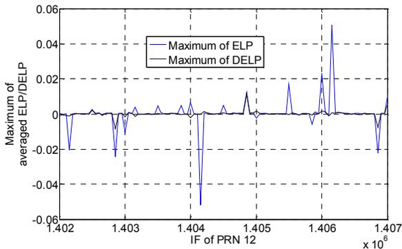
**Figure 13 – Comparison of maximum values of averaged ELP with that of DELP for PRN 12 in the presence of PRN 25 (IF=1405150 Hz) and multipath in PRN 25 signal with relative amplitude of 0.3 and phase difference of  $1.9672\pi$**
