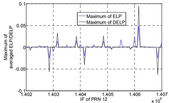
**Figure 11 – Comparison of maximum values of averaged ELP with that of DELP for PRN 12 in the presence of PRN 25 (IF=1405150 Hz) and multipath in PRN 25 signal with relative amplitude of 0.3 and phase difference of  $0.4918\pi$**
