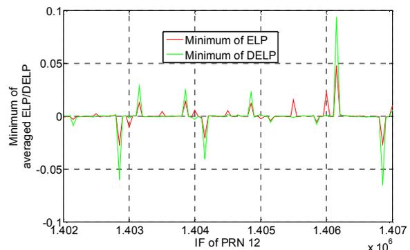
**Figure 12 – Comparison of minimum values of averaged ELP with that of DELP for PRN 12 in the presence of PRN 25 (IF=1405150 Hz) and multipath in PRN 25 signal with relative amplitude of 0.3 and phase difference of  $0.4918\pi$**
