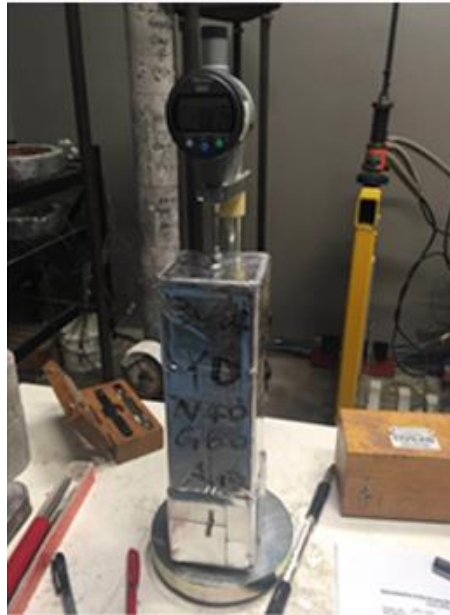
Figure 7 - 5: Autogenous shrinkage specimens.
