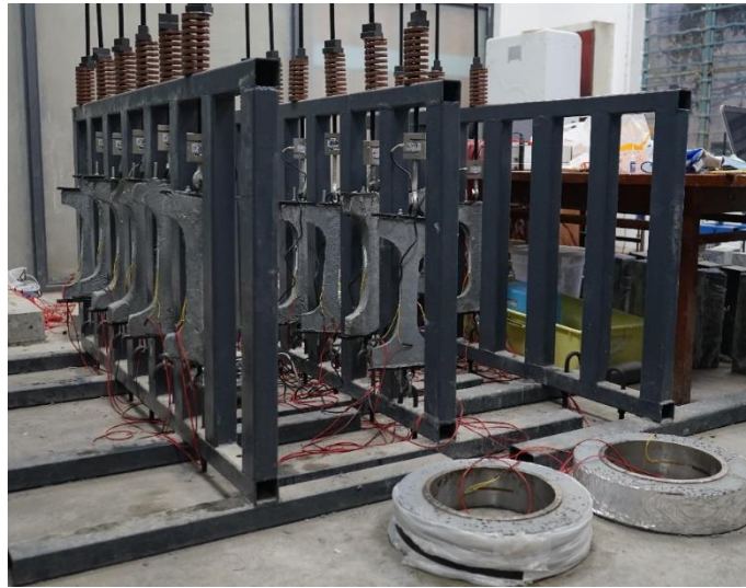
Figure 6 - 2: Tensile creep tests of UHPC.
