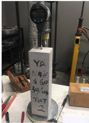
Figure 4 - 4: Total shrinkage specimens.
