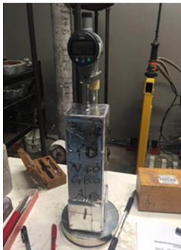
Figure 3 - 2: Autogenous shrinkage specimens.
