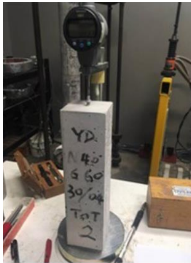
Figure 3 - 3: Total shrinkage specimens.
