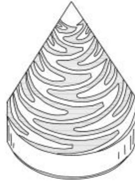
**Fig. 2** Conical sinuous antenna. (After Ref. [23])
