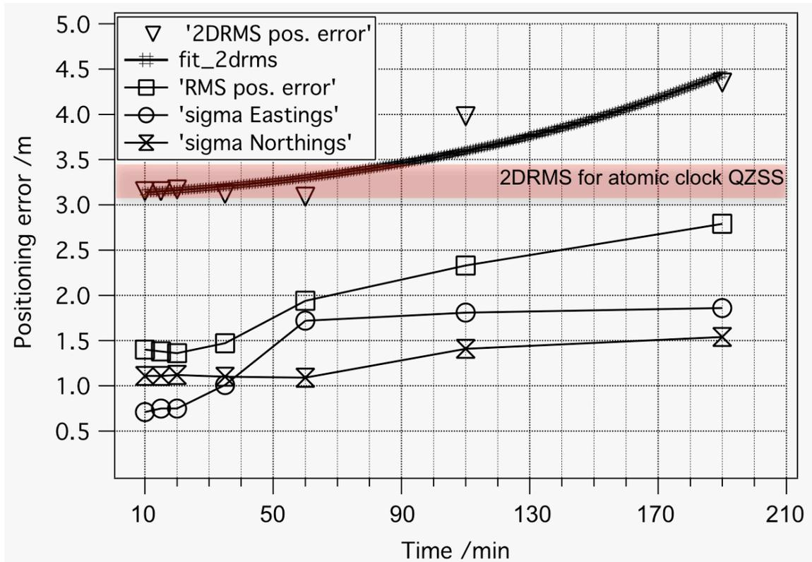
**Figure 3.** Positioning error, expressed as 2SRMS, RMS, Sigma Eastings and Sigma Northings, of the combined system GPS&QZSS when one of the QZSS clocks (VCXO) crosses the equatorial region and therefore is left in free running. The red area represents what the 2DRMS would be if all QZSS satellites were carrying ideal atomic references.
