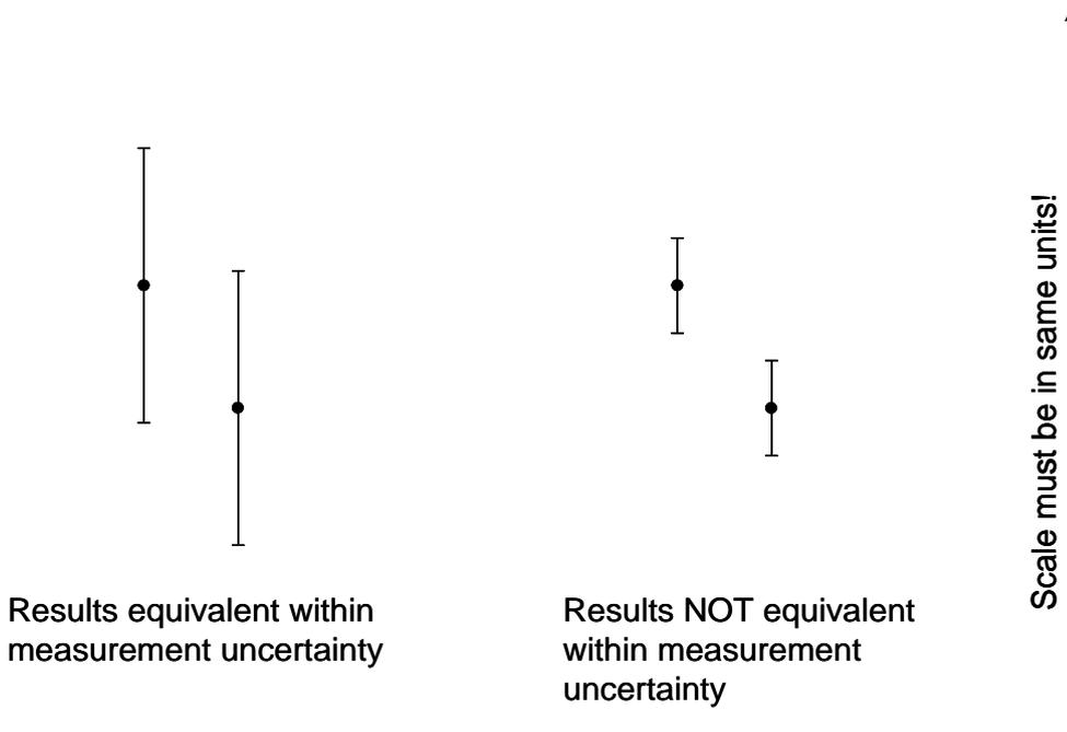
**Figure 4: Results, to be comparable, must be metrologically traceable to the same metrological reference, which implies that they have the same units. Comparison also requires measurement uncertainty.**
