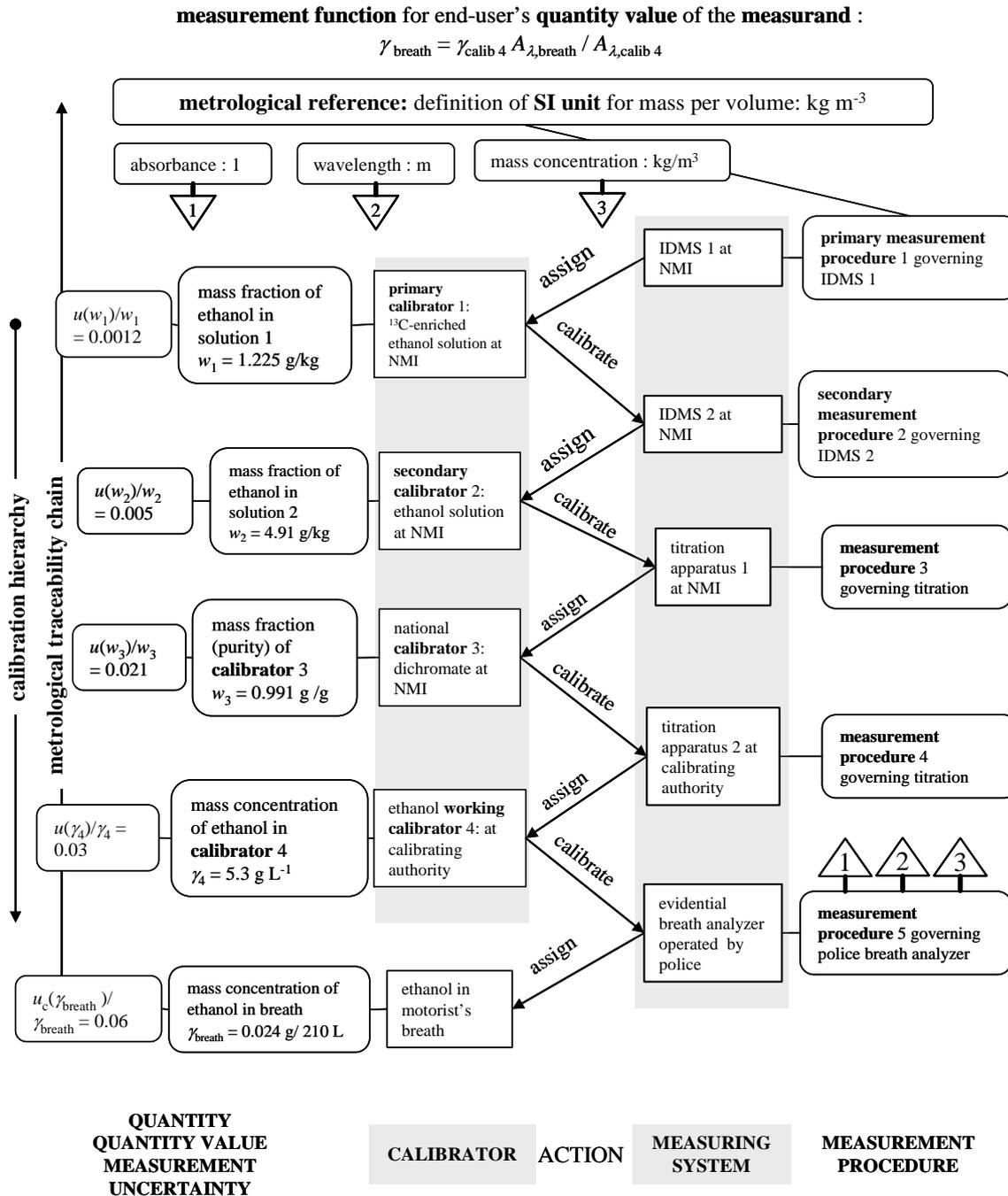
**Figure 6: Traceability chain for measurements of breath alcohol with calibration via dichromate titration. IDMS = isotope dilution mass spectrometry. Adapted from [3].**
