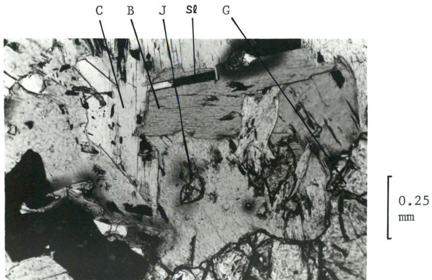
Fig. 4.14 Alteration of biotite (B) and gahnite (J) to chlorite (C), with sphalerite (S1) and garnet (G). (2/13C). PPL.
