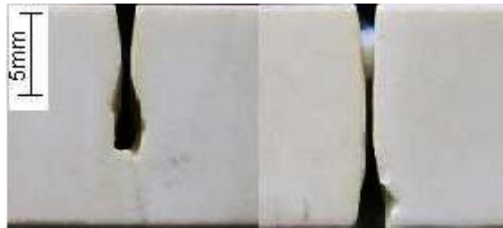
Figure 5. Samples of kerf profiles produced under normal cutting (left) and oscillation cutting (right): \dot{m}=9.1\text{g s}^{-1} , H=2\text{mm} , P=310\text{MPa} , u=1.33\text{mm s}^{-1} ; For oscillation cutting: \theta=8^\circ , F=10\text{Hz} .
