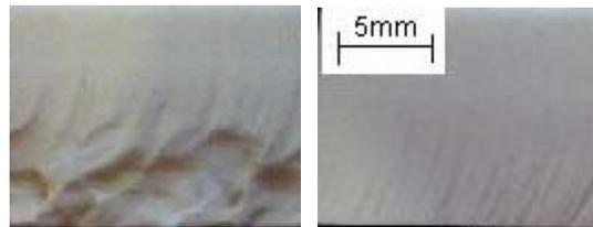
Figure 2. Samples of surfaces produced under normal cutting (left) and oscillation cutting (right):  $\dot{m} = 9.1 \text{ g s}^{-1}$ ,  $H = 4 \text{ mm}$ ,  $P = 380 \text{ MPa}$ ,  $u = 0.67 \text{ mm s}^{-1}$ ; For oscillation cutting:  $\theta = 4^\circ$ ,  $F = 14 \text{ Hz}$ .
