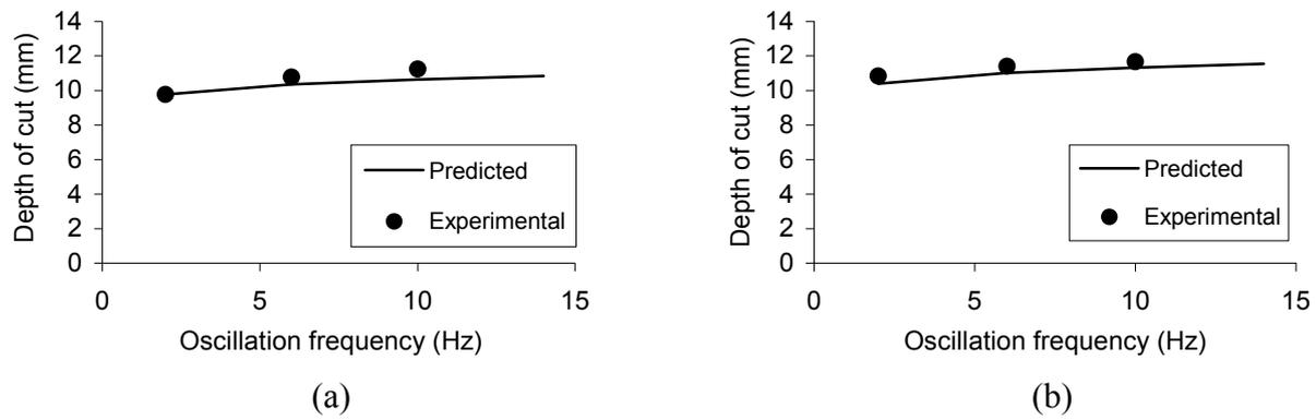
Figure 9. Comparisons between model predictions and experimental data: (a)  $\theta=4^\circ$ ,  $P=310\text{MPa}$ ,  $u=1.33\text{mm s}^{-1}$ ,  $H=3\text{mm}$ ,  $\dot{m}=11.3\text{g s}^{-1}$ . (b)  $\theta=2^\circ$ ,  $P=275\text{MPa}$ ,  $u=0.67\text{mm s}^{-1}$ ,  $H=2\text{mm}$ ,  $\dot{m}=6.8\text{g s}^{-1}$ .
