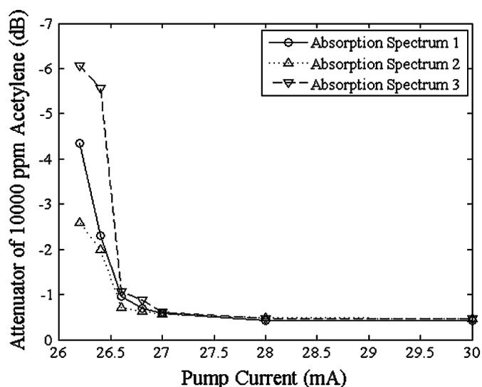
Fig. 3. Absorption intensity versus pump current.
