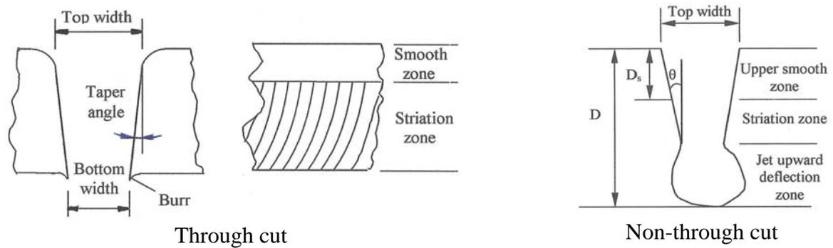
Fig. 1. Characteristics of kerfs produced by an AWJ.
