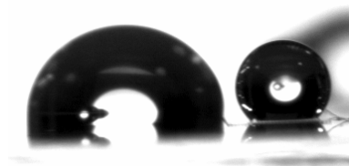
Figure 2: A droplet on a smooth PDMS surface, left and a patterned superhydrophobic surface, right.
