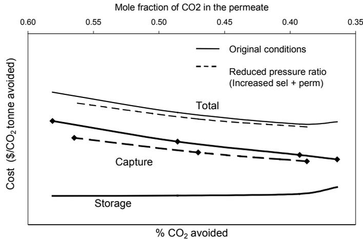
Figure 1. Change in cost for CO<sub>2</sub> capture with improved membrane selectivity and permeability
