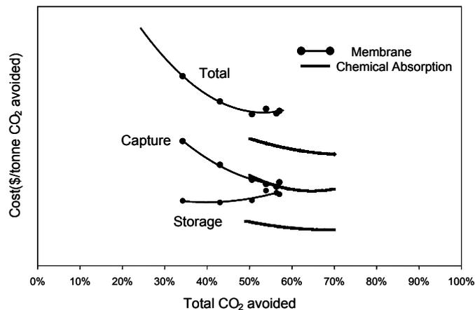
Figure 2: Costs of CO<sub>2</sub> capture, storage and sequestration (total) for different capture technologies
