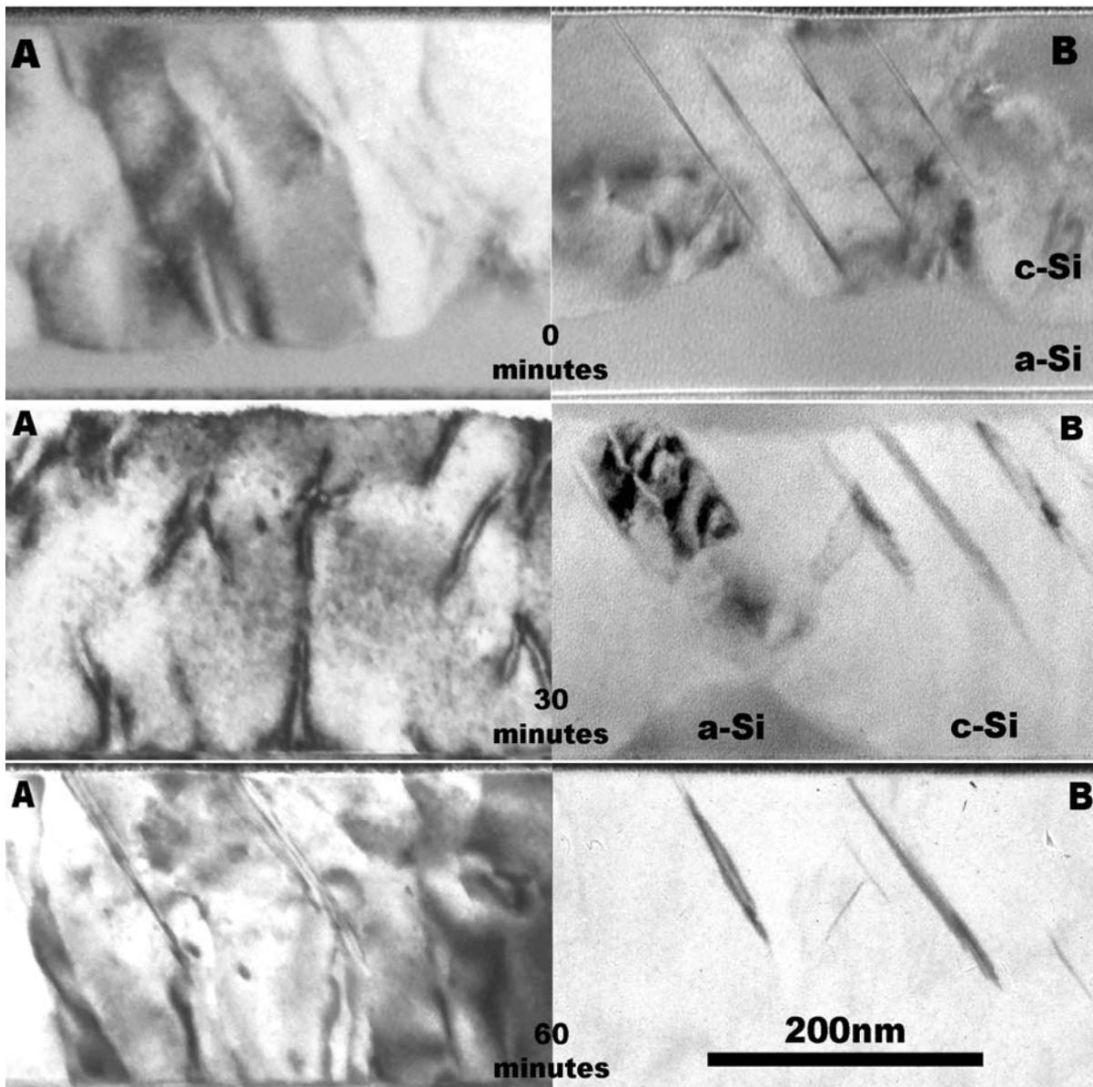
Figure 2: Bright field TEM images taken with a beam orientation parallel to: A  $\{200\}$  plane to highlight dislocations, labeled “A”, and a  $\{111\}$  plane to highlight planar faults, labeled “B”. Annealing times for each sample at 550°C are indicated. All samples are of the same magnification.
