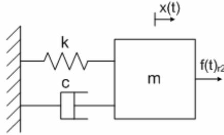
Figure 4 single degree of freedom blade model
