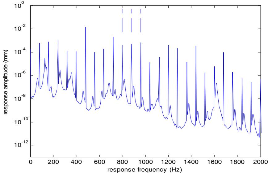
Figure 5 PSD of total casing response, vertical dashed lines at shaft speed spacing
