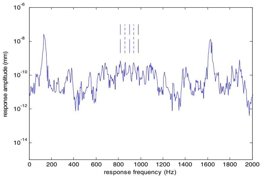
Figure 7 Cyclic spectrum at  $\alpha = 2(BPF + SPF)$ , vertical dashed lines at  $(4-6) \times$  shaft speed + blade natural frequency, vertical dotted lines at frequencies wrapped around zero.
