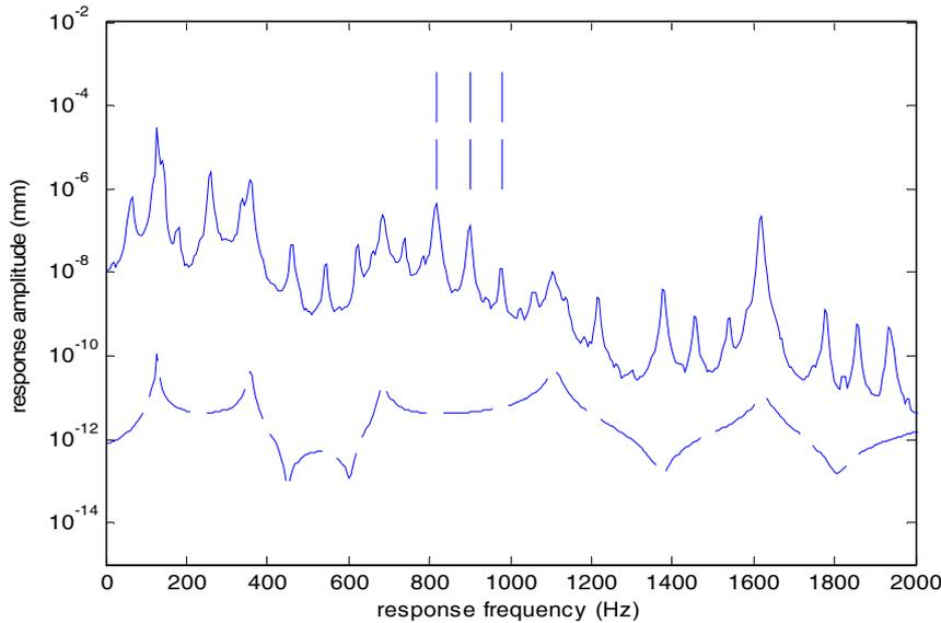
Figure 6 Residual PSD — , structural transfer function ---- , vertical dashed lines at  $(4-6) \times \text{shaft speed} + \text{blade natural frequency}$ .
