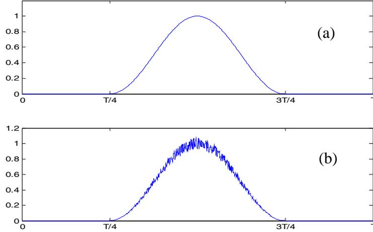
Figure 3 blade forcing function, purely deterministic (a), with random fluctuations (b)
