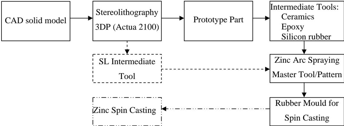
Fig. 2. Process chain for spin casting tooling.
