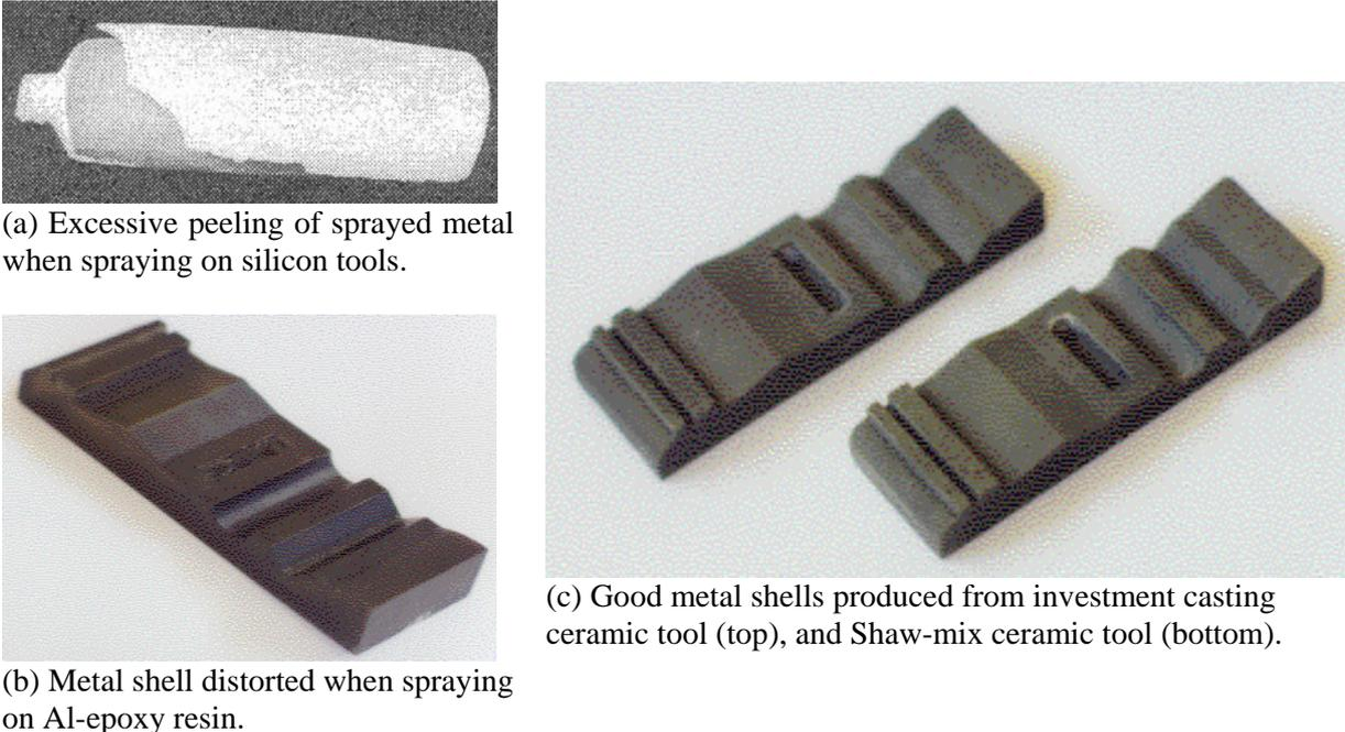
Fig. 6. Photographs of metal shells produced using different intermediate tools.
