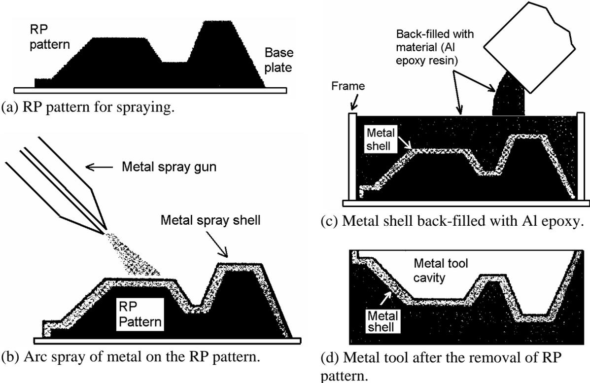
Fig. 4. The tool making process using arc metal spraying.
