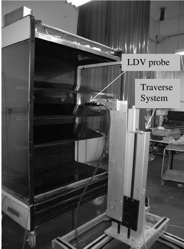
Fig. 4 Refrigerated Display Cabinets with Laser Doppler Velocimetry Probe
