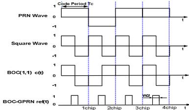
**Fig. 3** BOC(1,1) & reference wave of BOC-GPRN
