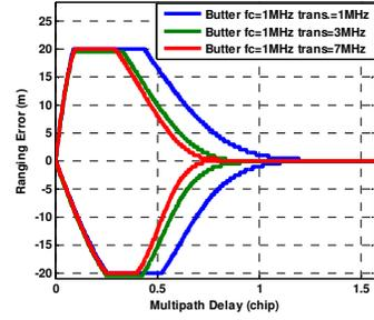
**Fig. 9** Multipath error increased as the filter transition BW decreased (Butterworth;  $W2=0.1\text{chip}$ )
