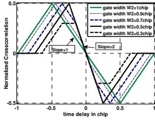
**Fig. 4** BOC-GPRN discriminators with infinite BW
