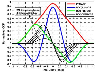
**Fig. 5** Pre-correlation filtering effects with 3MHz Passband BW 2MHz transition BW (Kaiser window)
