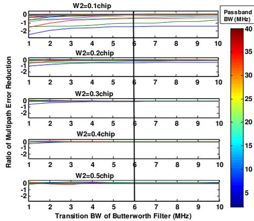
**Fig. 11** The ratio of differences between multipath error areas (Limited BW VS. Infinite BW)
