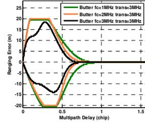
**Fig. 10** Multipath error increased as the filter passband BW decreased (Butterworth;  $W2=0.1\text{chip}$ )
