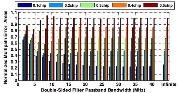
**Fig. 12** The normalized multipath error areas for BOC-GPRN discriminators (varying  $W2$  and Butterworth Filter BW, 6MHz Filter transition bandwidth.)
