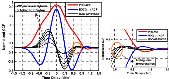
**Fig. 7** (In left) Ripple effects the pre-correlation filter. (Butterworth, GW=0.1chip,  $f_c=2\text{MHz}$   $f_s=3\text{MHz}$ )
