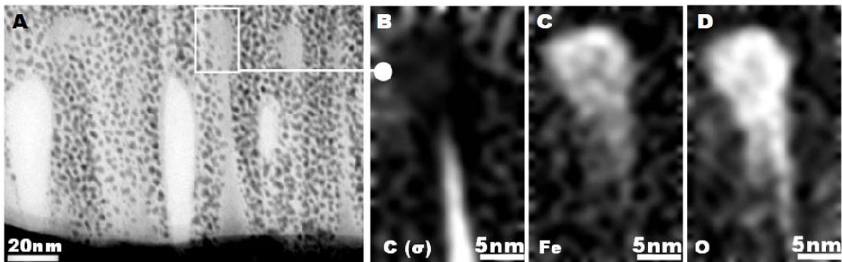
Fig. 4 (A) bright field STEM image of diamond nano-whiskers defining the areas for the EELS map for (B), (C) and (D). EELS maps corresponding to background subtracted signal integrals for; (B)  $\sigma$ -bonded carbon (diamond,  $\sim 35$  eV), (C) iron (L edge, 710 eV) and (D) oxygen (K edge  $\sim 540$  eV).
