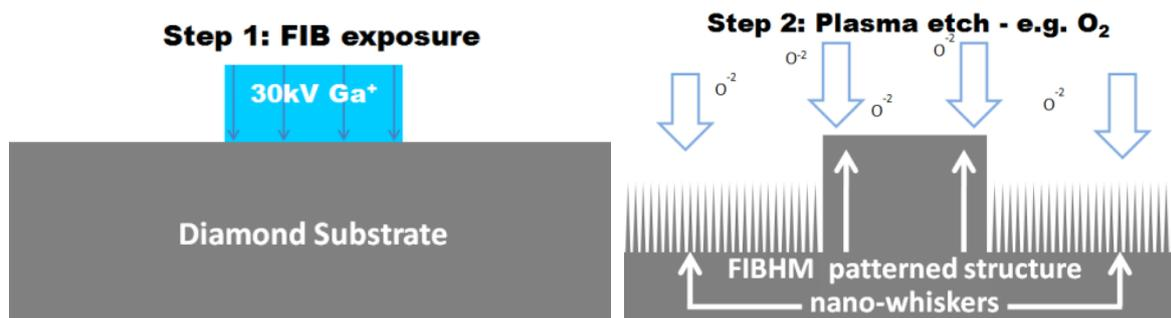
Fig. 1: The Focused Ion Beam Hard Mask technique: Step 1 is a local exposure of the diamond surface with a Ga<sup>+</sup> Focused Ion Beam microscope. Step 2 is a plasma etch of the diamond leaving the patterned areas raised as they have been masked from the etch by the FIBHM. Nano-whiskers can form around the un-exposed areas as indicated.
