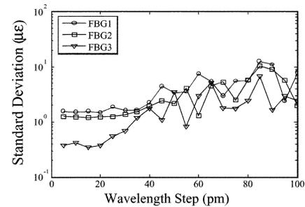
Fig. 5. Evolution of resolutions versus wavelength step. The width of the wavelength windows is fixed at 1600 pm.
