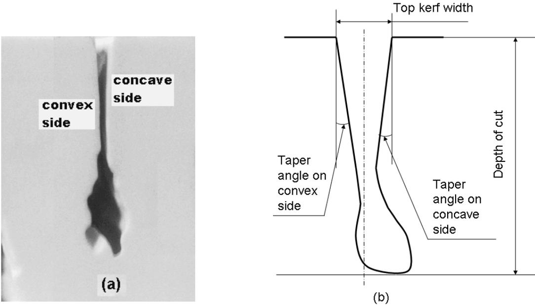
**Fig. 1** Typical kerf profile and geometrical definitions
