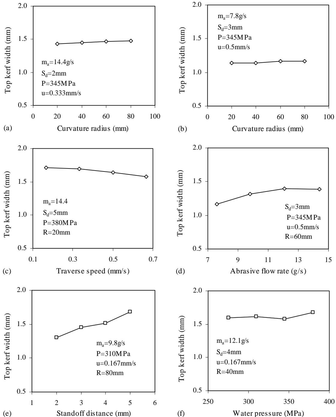
**Fig. 4** The effect of process parameters on the top kerf width.
