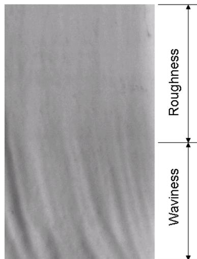
**Fig. 2** Characteristics of surfaces produced in AWJ profile cutting
