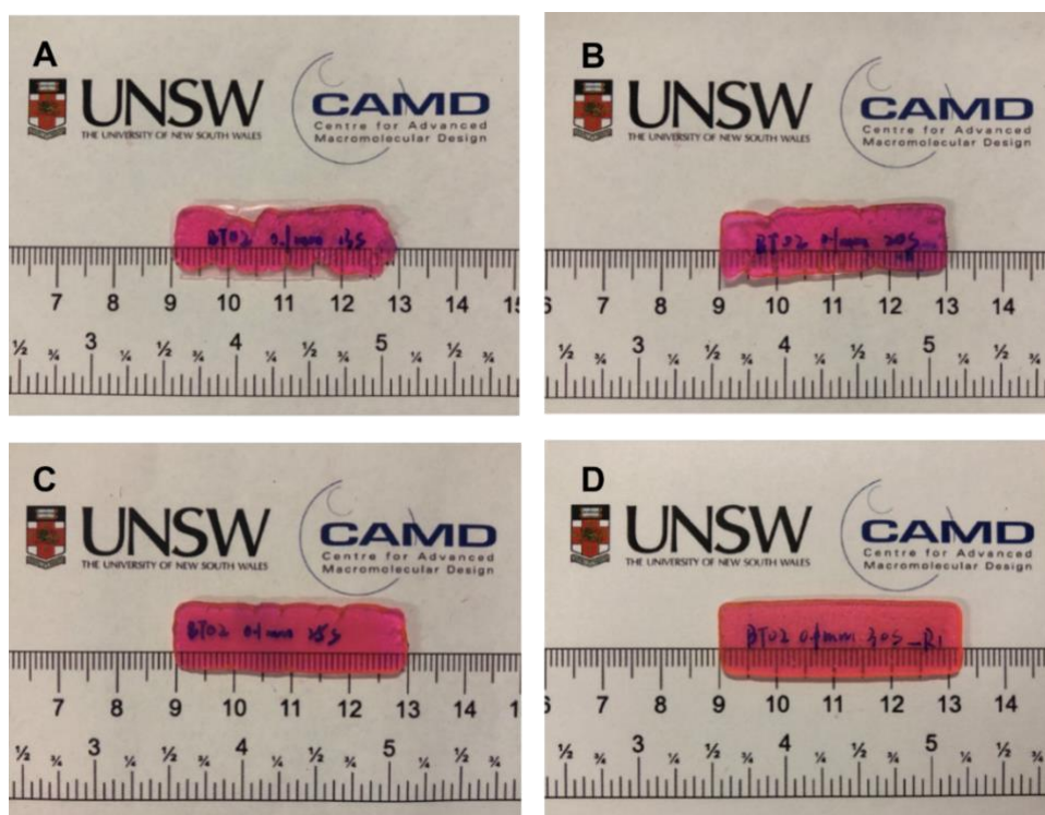
Figure 3.8 3D printed object definition using a 100 \mu\text{m} layer slicing thickness and various layer cure times with the resin formulation of [EB] : [DMAM] : [PEGDA] : [BTPA] : [TEtOHA] = 0.01 : 164 : 382 : 1 : 20 in bulk. (A) 13 s exposure time per layer; (B) 20 s exposure time per layer; (C) 25 s exposure time per layer; (D) 30 s exposure time per layer.
