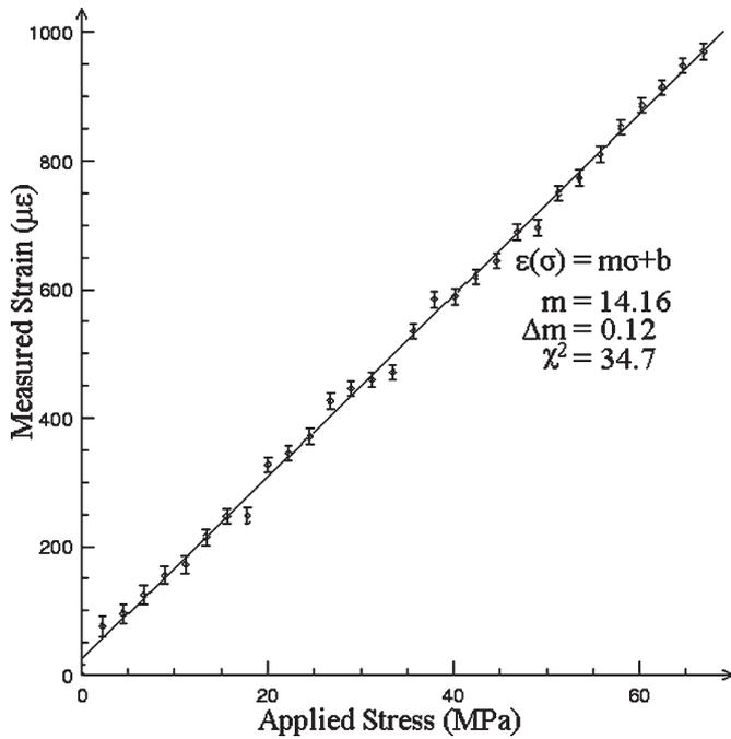
Fig. 4. Stress-strain relation for the  $j = 2.5$  channel.
