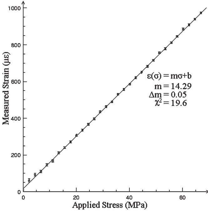
Fig. 2. Stress-strain relation for the  $j = 1$  channel.
