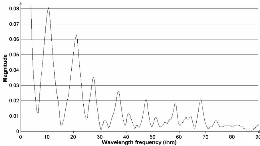
Figure 4. Fourier spectrum of 8 spectrally overlapping carrier modulated FBG sensors with first order compensation for spectral shadowing.
