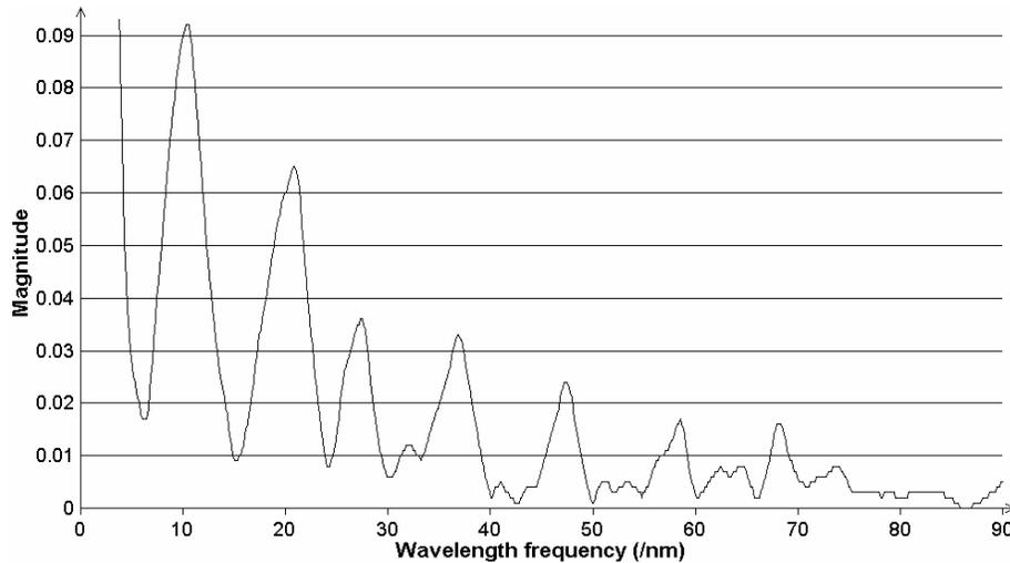
Figure 5. Fourier spectrum of 8 spectrally overlapping carrier modulated FBG sensors with full compensation for spectral shadowing and multiple reflections.
