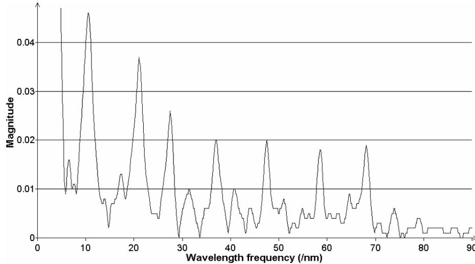
Figure 3. Fourier spectrum of 8 spectrally overlapping carrier modulated FBG sensors with no compensation for spectral shadowing or multiple scattering.
