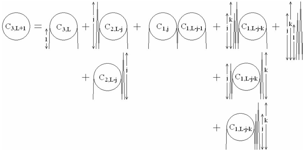
Figure 2. Scattering processes contributing to 3<sup>rd</sup> order multiple reflections in a series array of identical sensors.
