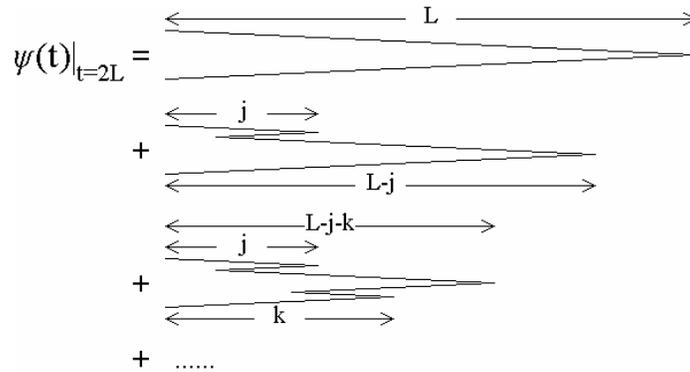
Figure 1. Signals from various paths that reach the detector at the same normalised time (2L) in a TDM sensor system.
