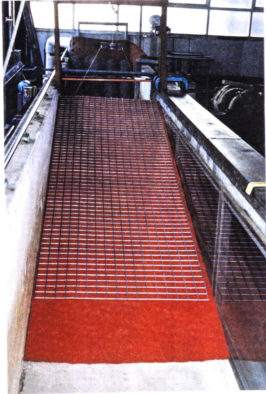
Photo 1 - The permeable sloping absorber after installation
