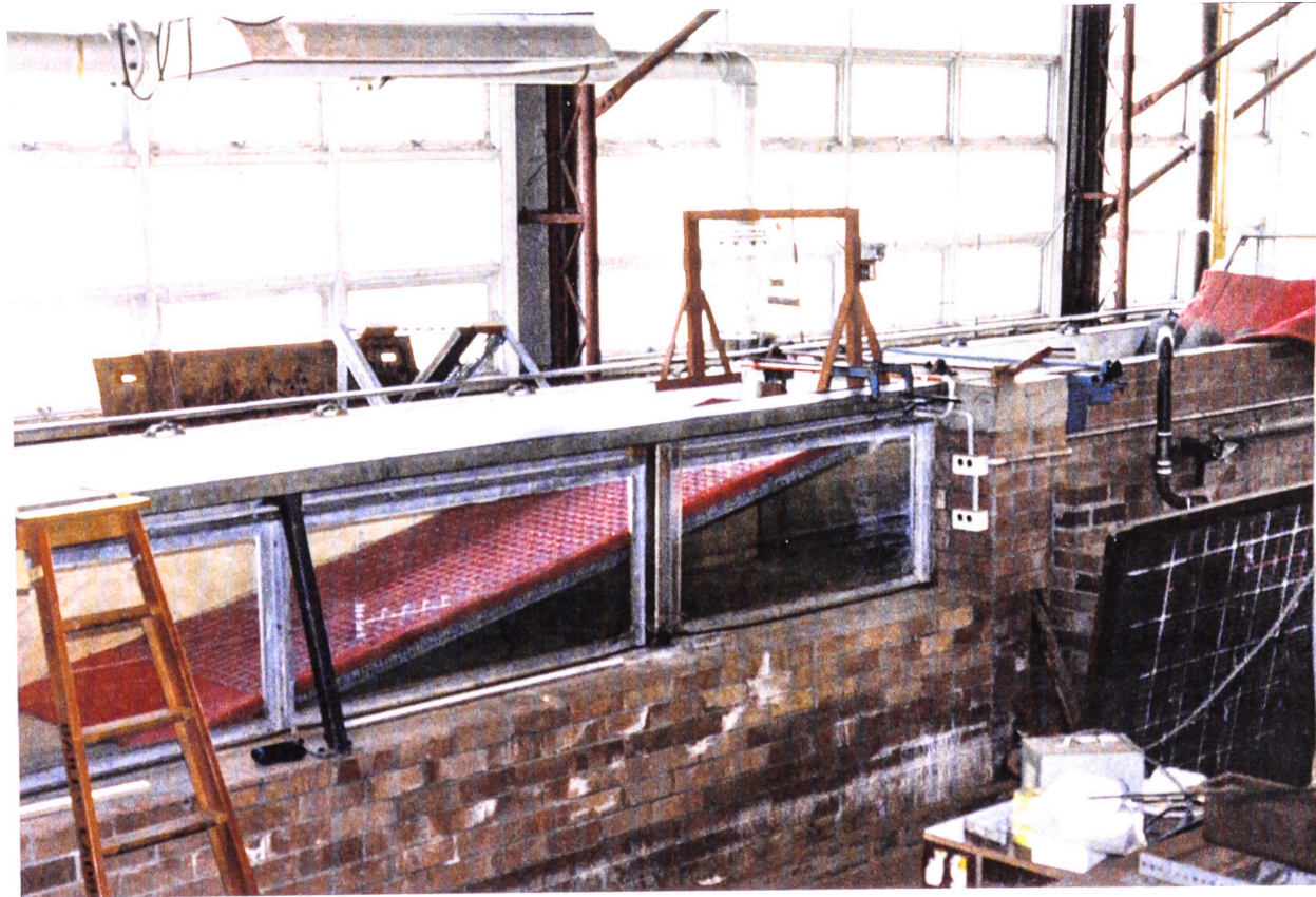
Photo 3 - View of the permeable sloping absorber installed in the shallow water part of the wave flume
