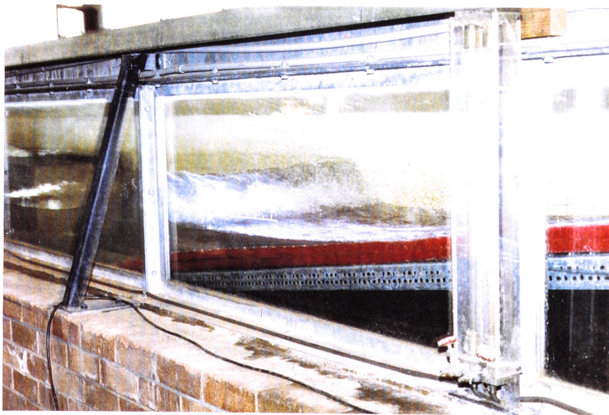
Photo 5 - Breaking of waves in front of the wave absorber
