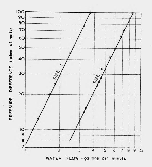
UNIVERSITY OF NEW SOUTH WALES THE RESEARCH WATER LABORATORY Date: 18 - 4 - 61 VENTURI METER CHARACTERISTICS Drawn D. T. Howell CE-E-2327 PATTERN - SIZES | & 2 ADMIRALTY P.A Traced D.T.H Checked
