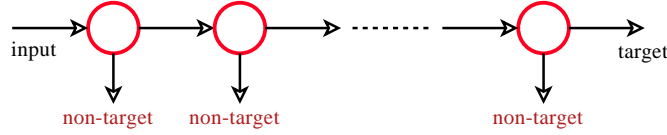
Figure 4.1: An illustration of cascade classifiers. Here a circle represents a node classifier. An input patch is classified as a target only when it passes tests at all node classifiers.
