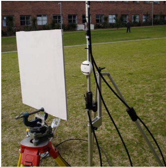
Figure 13: Plasterboard sheet blocking LL2
