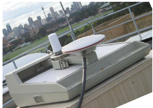
Figure 8: HP XY plotter table with Locata and Leica AT502 antennas
