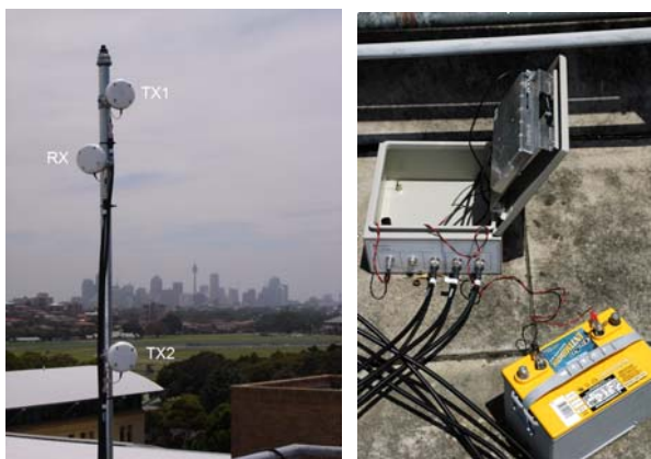
Figure 2: LocataLite (LL5) antenna setup (left) and weatherproof enclosure (right)
