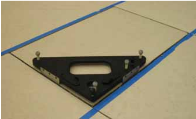
Figure 3.1 L-Frame device for static calibration
