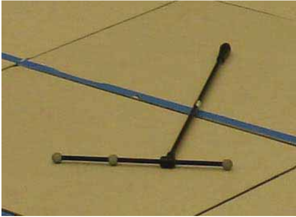
Figure 3.2 240mm Space Bar Wand device for dynamic calibration
