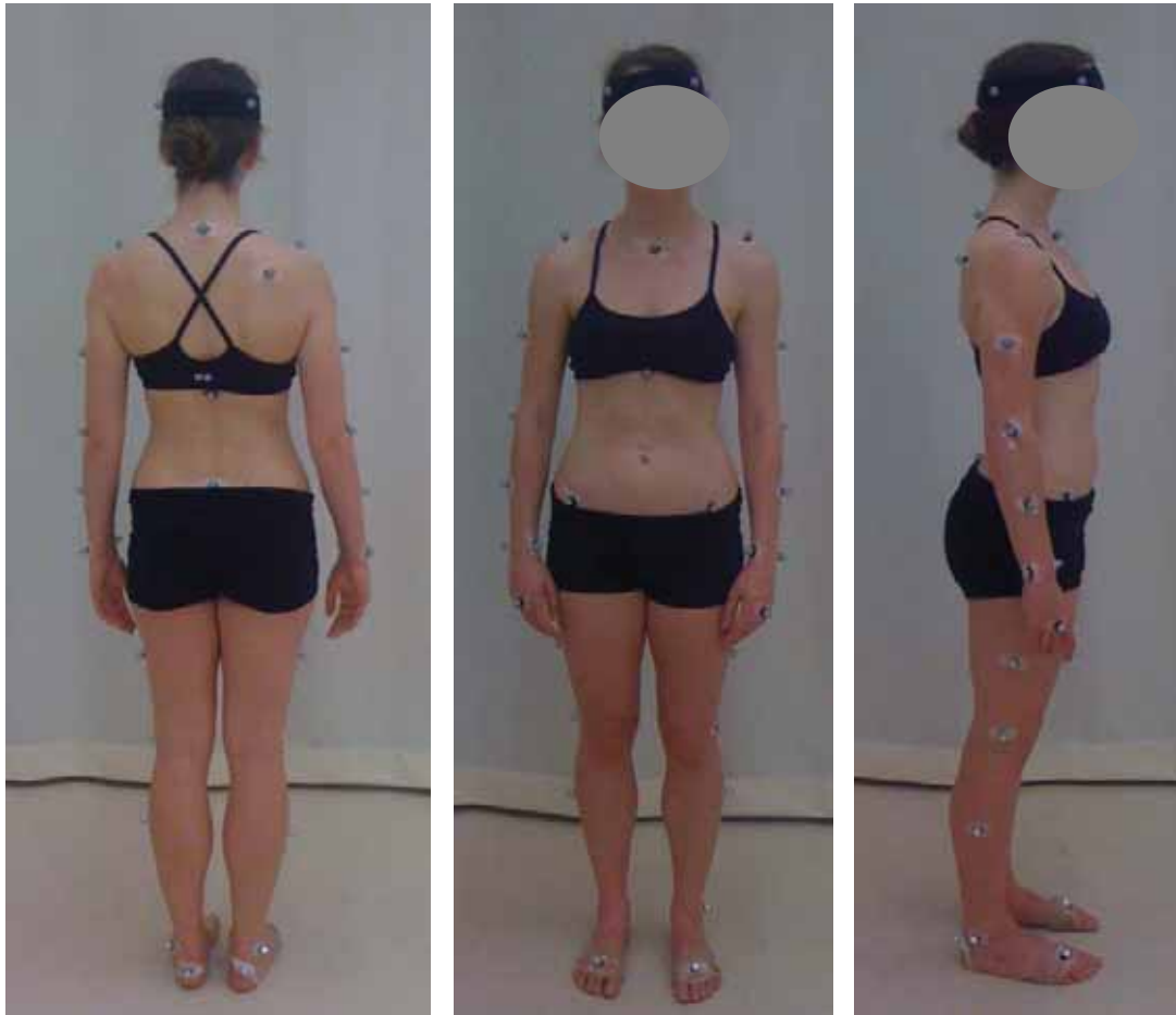
Figure 3.4 Reflective marker placement on participant
