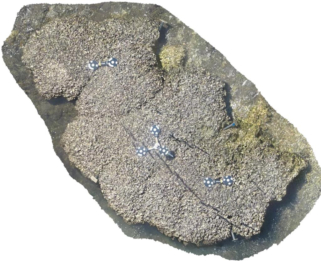
Figure B.2. Top-view of a three-dimensional mesh model of Crookhaven River Reef 4 captured from AgiSoft PhotoScan Professional (2015, v1.1.6) Agisoft LLC, Russia. Triax scale feature can be seen in the middle of the reef model while dumbbell scale features are observed in the top and bottom side of the model.
