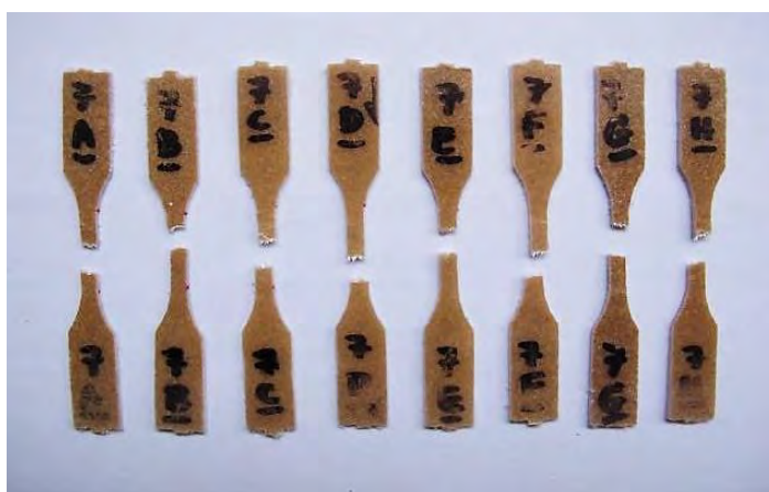
Figure V.7: Tensile specimens of hot pressed extruded UKF/HDPE composites (UKF/HDPE_H) strip after testing.
