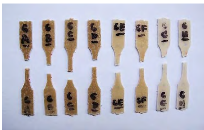
Figure V.9: Tensile specimens of hot pressed extruded KFTHA/HDPE (KFTHA/HDPE_H) strip after testing.
