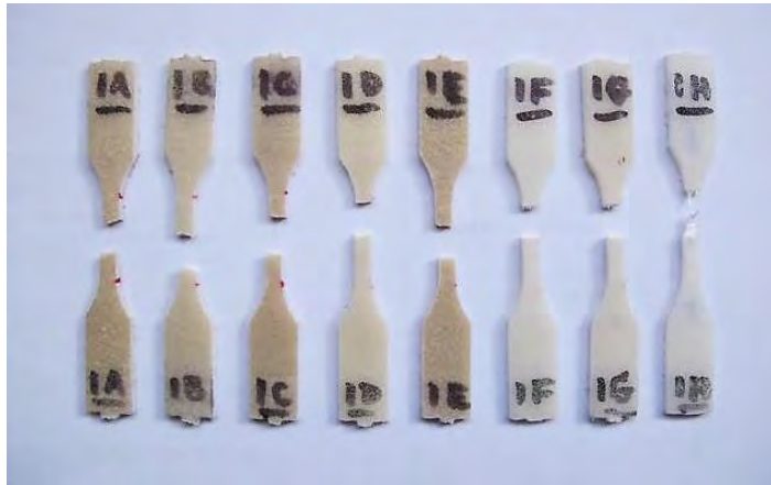
Figure V.4: Tensile specimens of extruded KFTHA/HDPE strip after testing.
