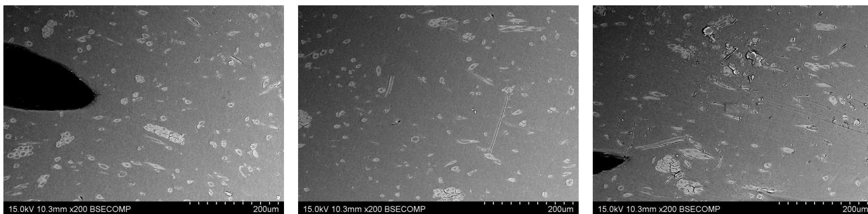
Figure X.26: SEM micrographs of transverse section of KFTN/HDPE_H strip composite (Sample no. 2 (8C)).
