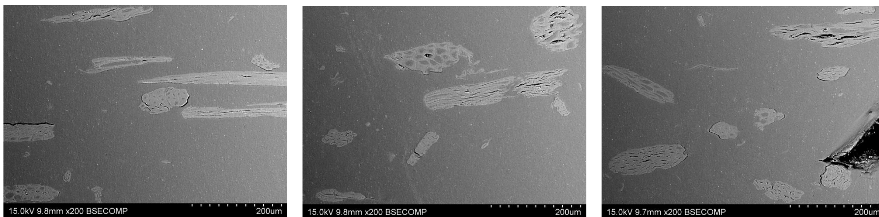
Figure X.24: SEM micrographs of transverse section of UKF/HDPE_H strip composite (Sample no. 3 (7D)).
