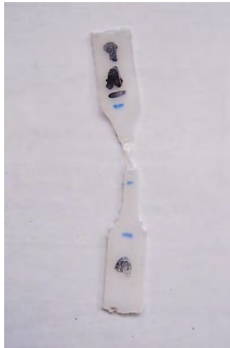
Figure V.1: Tensile specimens of extruded HDPE strip after testing.
