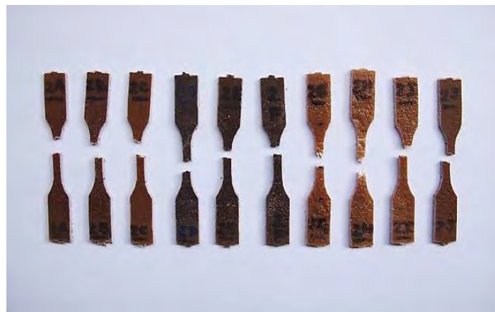
Figure V.3: Tensile specimens of extruded KFTN/HDPE strip after testing.
