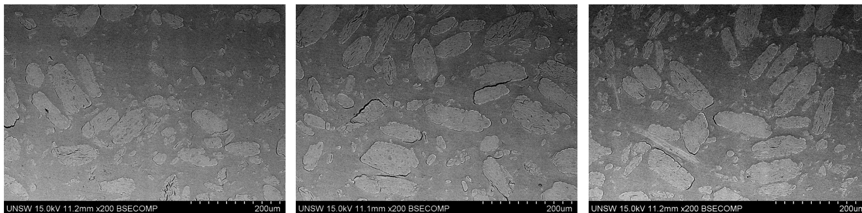
Figure X.1: SEM micrographs of transverse section of UKF/HDPE rod composite (Sample no. 1 and End A).
