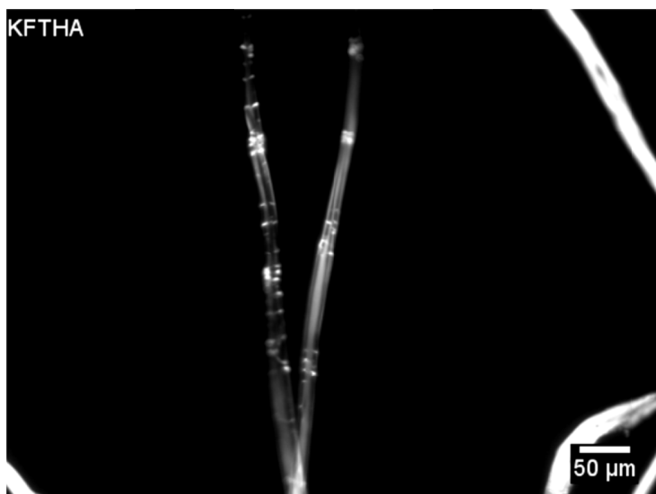
Figure 3.36: Cross-polarised light micrograph of KFTHA2 fibres showing nodes and dislocations.
