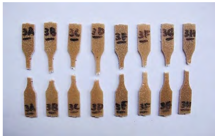
Figure V.2: Tensile specimens of extruded UKF/HDPE strip after testing.
