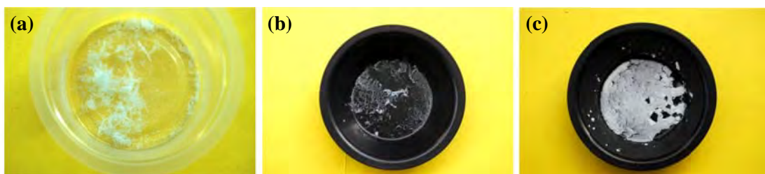
Figure 3.9: KFTN fibres (a) air-dried, (b) freeze-dried (low fibre to water ratio) and (c) freeze-dried (high fibre to water ratio).
