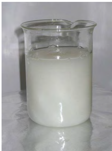
Figure I.9: \alpha -cellulose immersed in a mixture of \text{H}_2\text{O}_2 and \text{CH}_3\text{COOH} .
