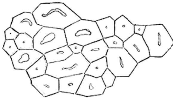
Figure 5.5: Schematic diagram of cross-section of a flax technical fibre (Baley, 2002).
