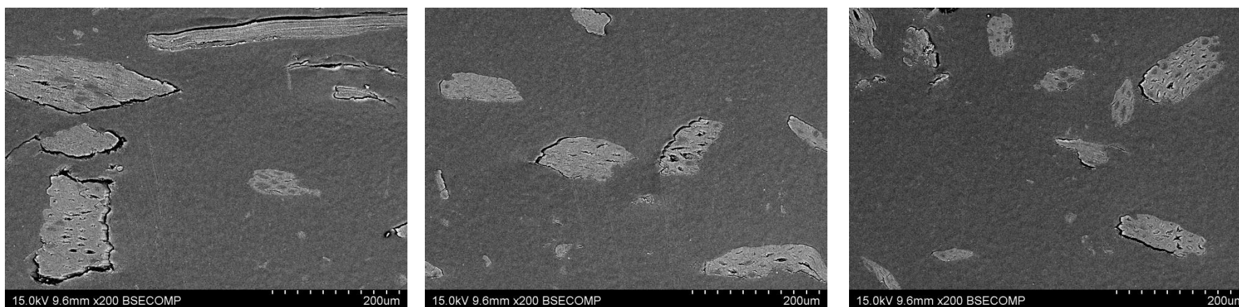
Figure X.14: SEM micrographs of transverse section of UKF/HDPE strip composite (Sample no. 2 (3D)).
