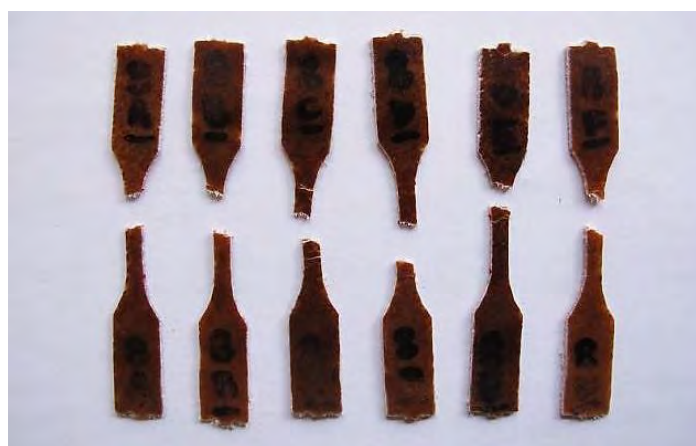
Figure V.8: Tensile specimens of hot pressed extruded KFTN/HDPE (KFTN/HDPE_H) strip after testing.
