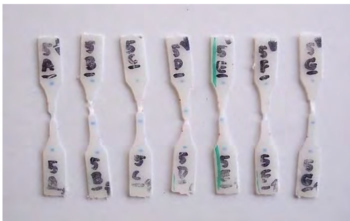
Figure V.6: Tensile specimens of hot pressed extruded HDPE/MAPE (HDPE/MAPE_H) strip after testing.
