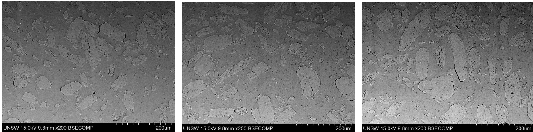
Figure X.4: SEM micrographs of transverse section of UKF/HDPE rod composite (Sample no. 2 and End B).
