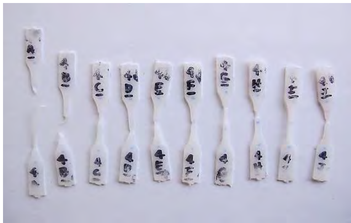
Figure V.5: Tensile specimens of hot pressed extruded HDPE (HDPE_H) strip after testing.
