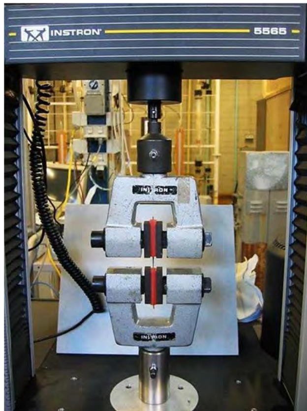
Figure 4.7: Setup using silicone rubber strip fixtures for tensile testing of an extruded composite rod using an Instron universal testing machine.
