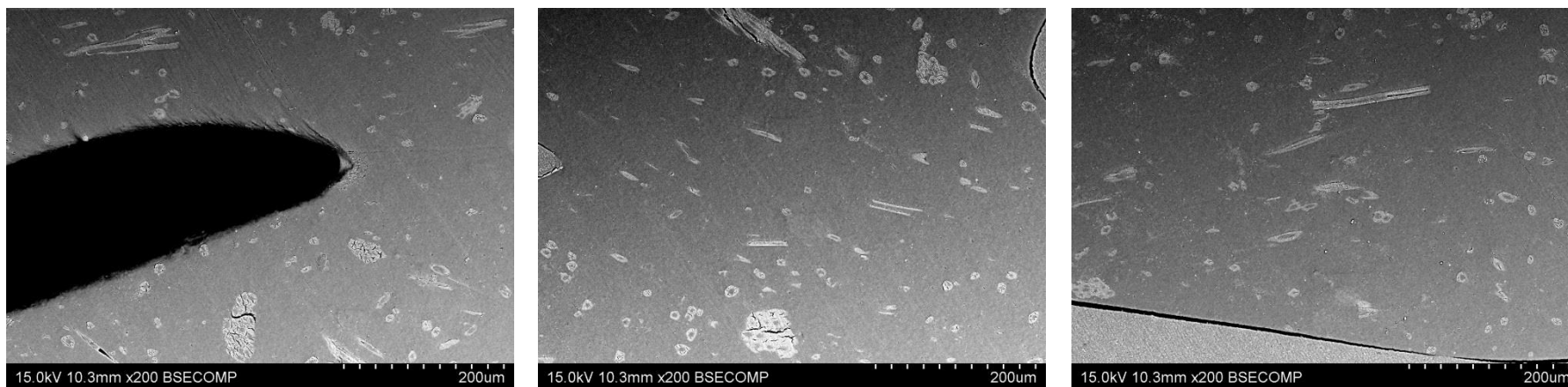
Figure X.25: SEM micrographs of transverse section of KFTN/HDPE_H strip composite (Sample no. 1 (8A)).
