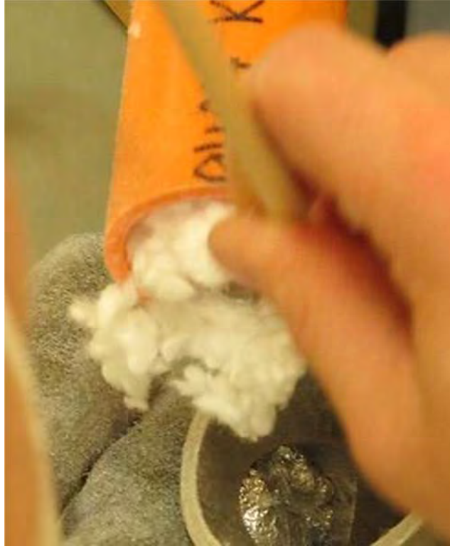
Figure 4.64: KFTHA fibres fed into a hopper of a twin-screw extruder.
