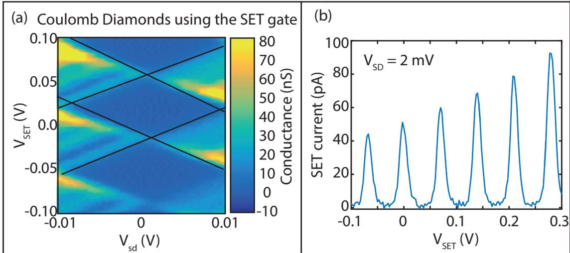
Figure 4.9: Electrical characterization of the ALD-SET device using the in-plane gate voltage  $V_{SET}$ . (a) The quantum dot conductance plotted as a function of source-drain bias voltage  $V_{sd}$  and the SET gate voltage. Coulomb blockade is observed with a constant charging energy of  $\approx 7.748 \pm 0.0683$  mV. (b) Coulomb peaks are measured in this experiment by varying the gate voltage for a fixed source drain bias of 2 mV.
