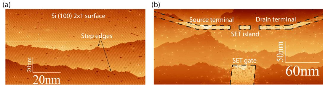
Figure 4.4: Fabrication of a STM based donor quantum dot device. (a) Hydrogen terminated Si (001) surface in the STM chamber before performing lithography. (b) A 3 terminal device consisting of source, drain and a gate patterned using the tip of the STM by selectively desorbing hydrogen from areas of interest. Source and drain terminals in this device are tunnel coupled to the SET island, while the gate is  $\sim 85$  nm away and is capacitively coupled to the SET island.
