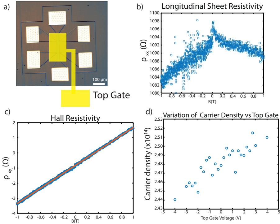
Figure 4.3: Characterization of Si:P  $\delta$ -layer with a metallic top patterned gate on an  $\text{Al}_2\text{O}_3$  dielectric. (a) Optical image of the Hall bar with the location of patterned top gate shown in yellow. (b) Longitudinal sheet resistivity of the Hall bar for a top gate voltage of 2 V. (c) Hall resistivity of the Hall bar for a top gate voltage of 2 V. (d) Variation of the carrier density with top gate voltage measured between -4 V to 4 V.
