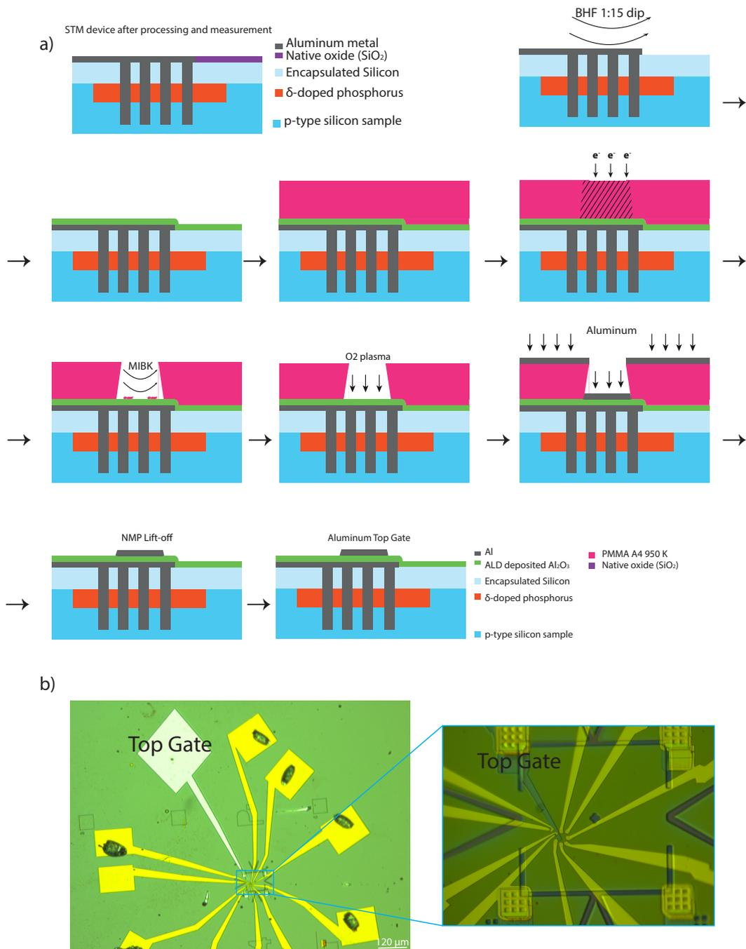
Figure 4.20: Integration of top gate on a 4 quantum dot STM patterned device . (a) Full processing recipe for patterning a top gate over STM fabricated devices. Note: These devices have native oxide present over the inner device structures, which is later removed when a BHF dip is performed. (b) Optical image showing the top gate along with the ohmics with the close-up image confirming that the position of the top gate is directly on top of the inner device structures which is crucial.
