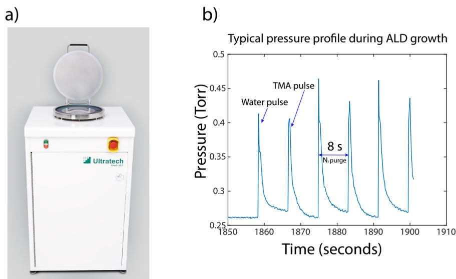
Figure 2.16: a) ALD reactor Savannah S200 by Cambridge Nanotech. Figure adapted from [120]. b) A typical pressure profile during growth of ALD based  $\text{Al}_2\text{O}_3$  using TMA and  $\text{H}_2\text{O}$  as precursors. Purge time during the run is set to 8 seconds using  $\text{N}_2$  gas. Base pressure during growth is 0.26 Torr.
