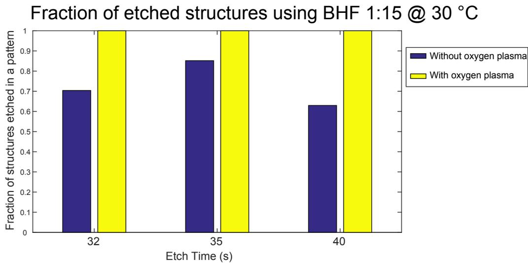
Figure 3.9: Bar graph showing the success rate in etched structures without (purple) and with (yellow) oxygen plasma for 32 seconds, 35 seconds and 40 seconds, respectively using a BHF 1:15 solution.
