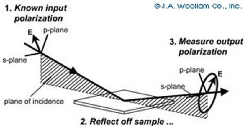
Figure 2.20: Schematic of Ellipsometry process [128]
