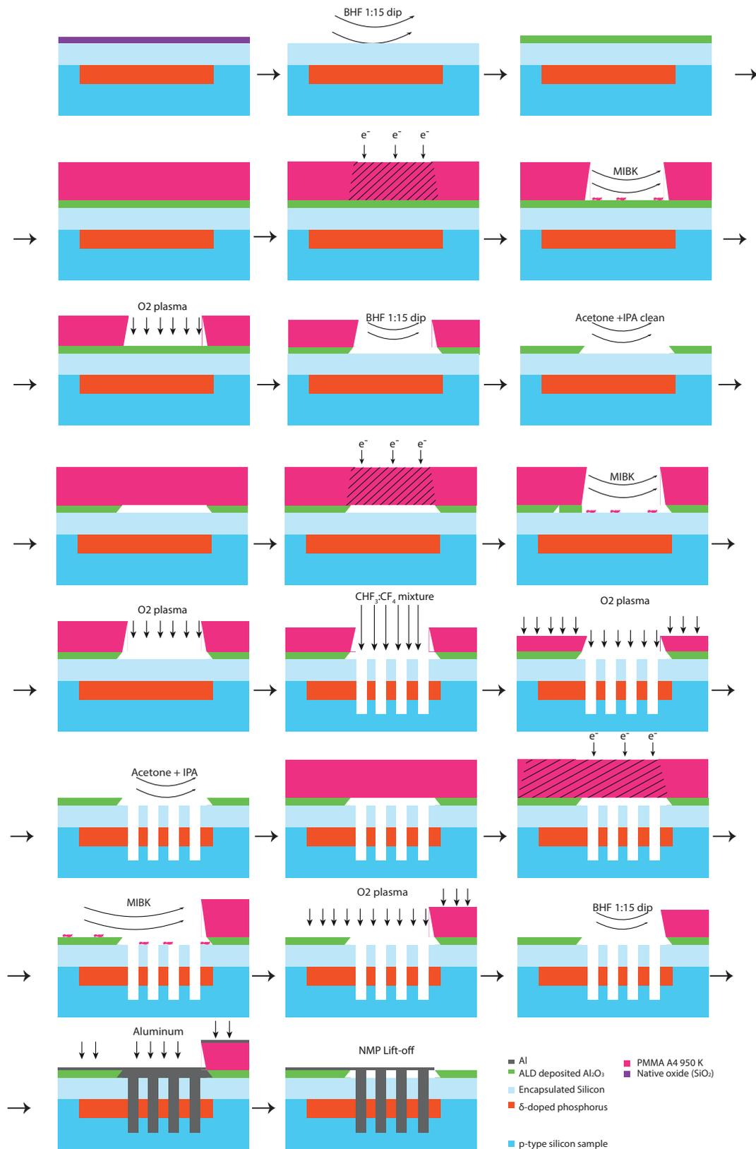
Figure 4.6: Process flow for adding a layer of  $\text{Al}_2\text{O}_3$  dielectric and then establishing ohmic contact to the buried Si:P device.
