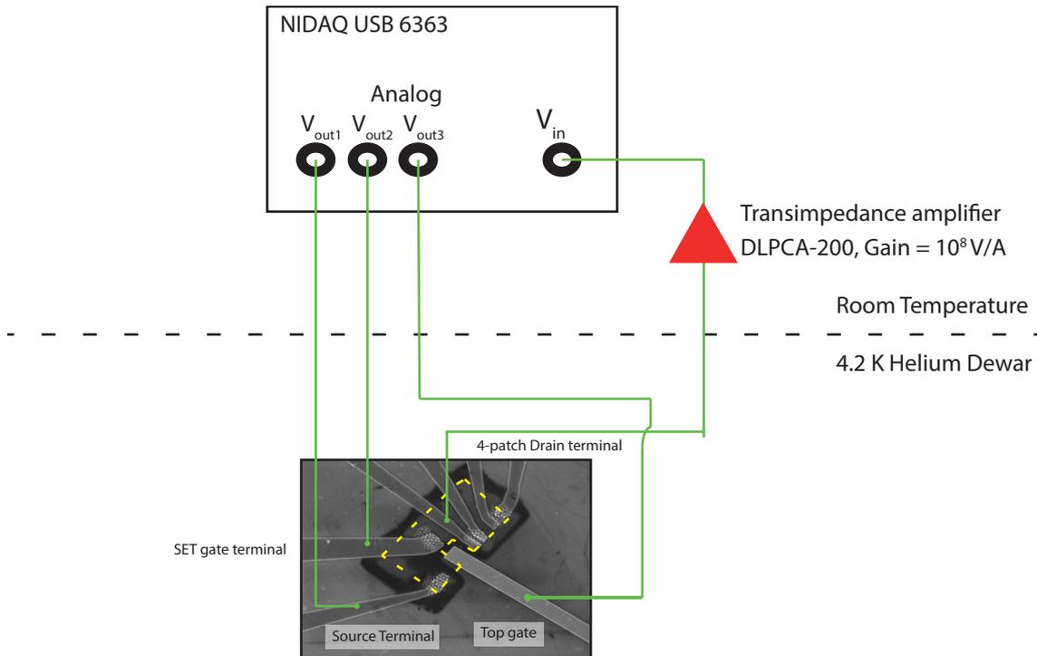
Figure 4.8: Measurement setup used in electrical characterization of the ALD-SET device. Analog voltage is applied through NIDAQ 6363 and output drain current is digitized using the same device after room temperature amplification using a Femto DLPCA-200 transimpedance amplifier with a gain of  $10^8$  V/A.
