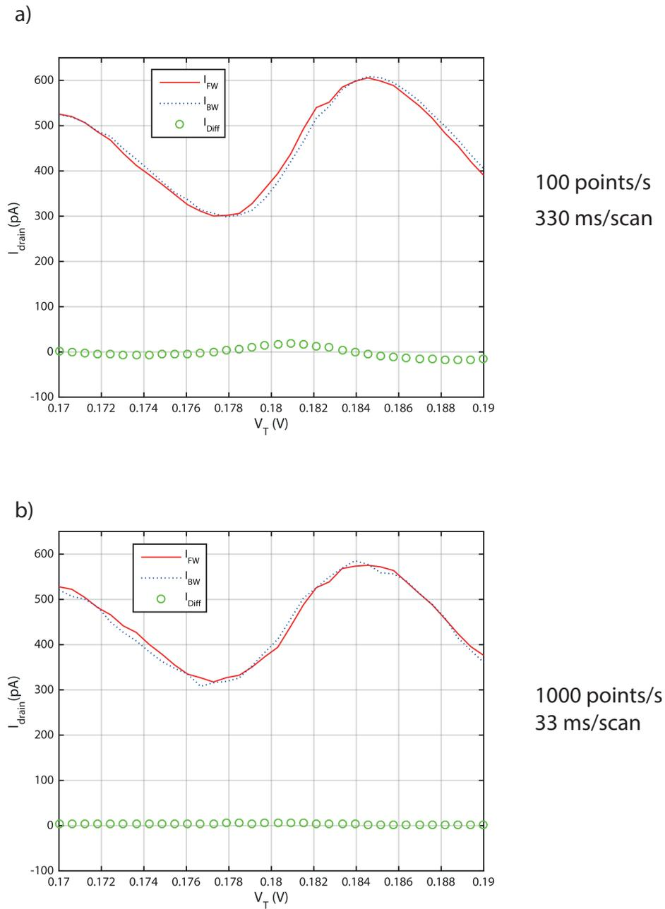
Figure 4.15: Forward and backward drain current shown using red and dashed blue lines is recorded for sweeping the top gate voltage back and forth once. Difference between the mean values of the forward and backward current (obtained after continuously scanning the gate voltage forward and backward) is shown using green bubbles. (a) Scan obtained for a data rate of 100 points/s (measured for 1 hour). (b) Scan obtained for a data rate of 1000 points/s (measured for 1 hour).
