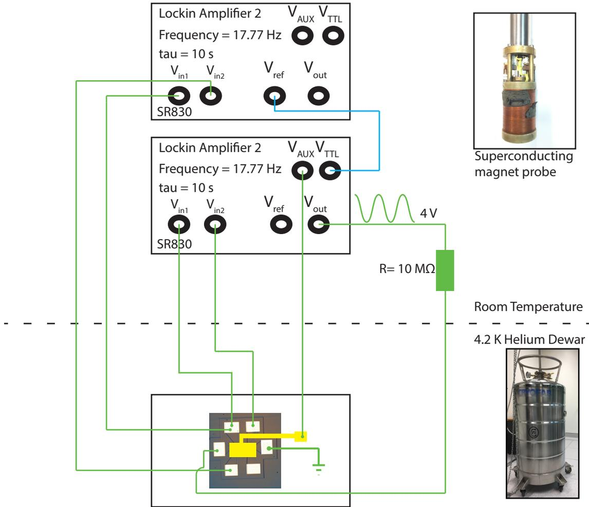
Figure 4.2: Electrical measurement configuration of the Hall bar consisting primarily of two lock-in amplifiers with their main settings depicted in the sketch using a frequency of 17.77 Hz and  $\tau = 10$  s (time constant). All measurements have been performed in a Helium dewar at 4.2 K (depicted in the bottom right inset). A photography of the superconducting magnet probe is shown in the top right inset.
