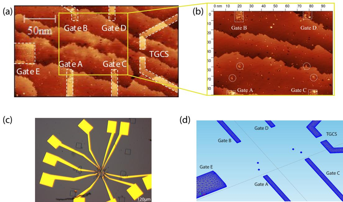
Figure 4.17: 4 STM-patterned donor dots in a coupled singlet-triplet architecture. (a) Overview of the 4-dot device. (b) Close-up of the 4-dot device showing the inner device dimensions containing all the four dots. (c) Optical image showing all the ohmic contacts patterned to establish contact with the buried phosphorus doped nanostructures. (d) COMSOL model showing the patterned 4-dot device.
