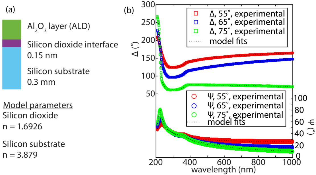
Figure 3.1: Ellipsometry measurements of Al<sub>2</sub>O<sub>3</sub> layers. (a) Layered model of deposited thin film on bare silicon substrate. (b) Data obtained from the ellipsometer after spectroscopy performed at 55°, 65° and 75°. Plot shows  $\psi$  and  $\Delta$  plotted for different detection wavelengths.
