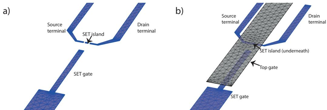
Figure 4.7: Schematic of ALD SET device in COMSOL. a) ALD SET device in a meshed configuration. b) ALD SET device patterned with a top gate in a meshed configuration.
