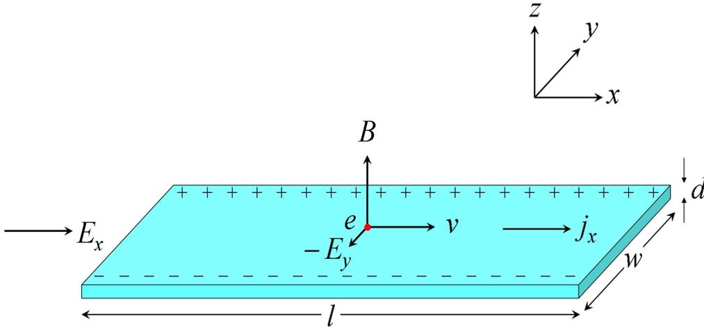
Figure 2.5: Classical Hall effect for a 2D system. Figure adapted from [34].
