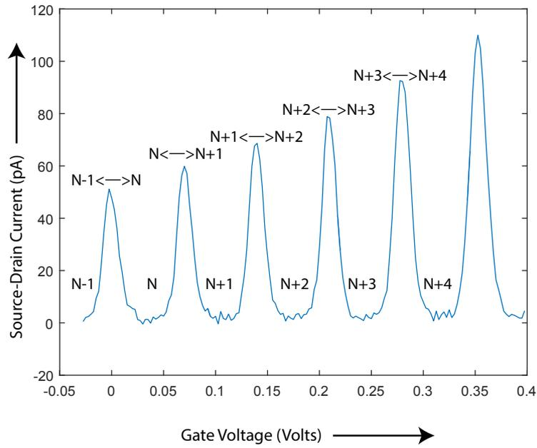
Figure 2.11: Experimental observation of Coulomb peaks observed in a STM patterned quantum dot with a charging energy of  $\sim 10$  meV. The figure shows periodic Coulomb peaks where each valley corresponds to the addition of an electron to the quantum dot by varying the gate voltage.
