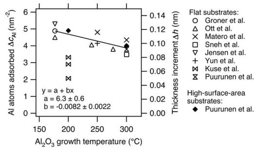
Figure 2.19: GPC in the ALD growth of aluminum oxide in steady growth regime. Figure adapted from [7].
