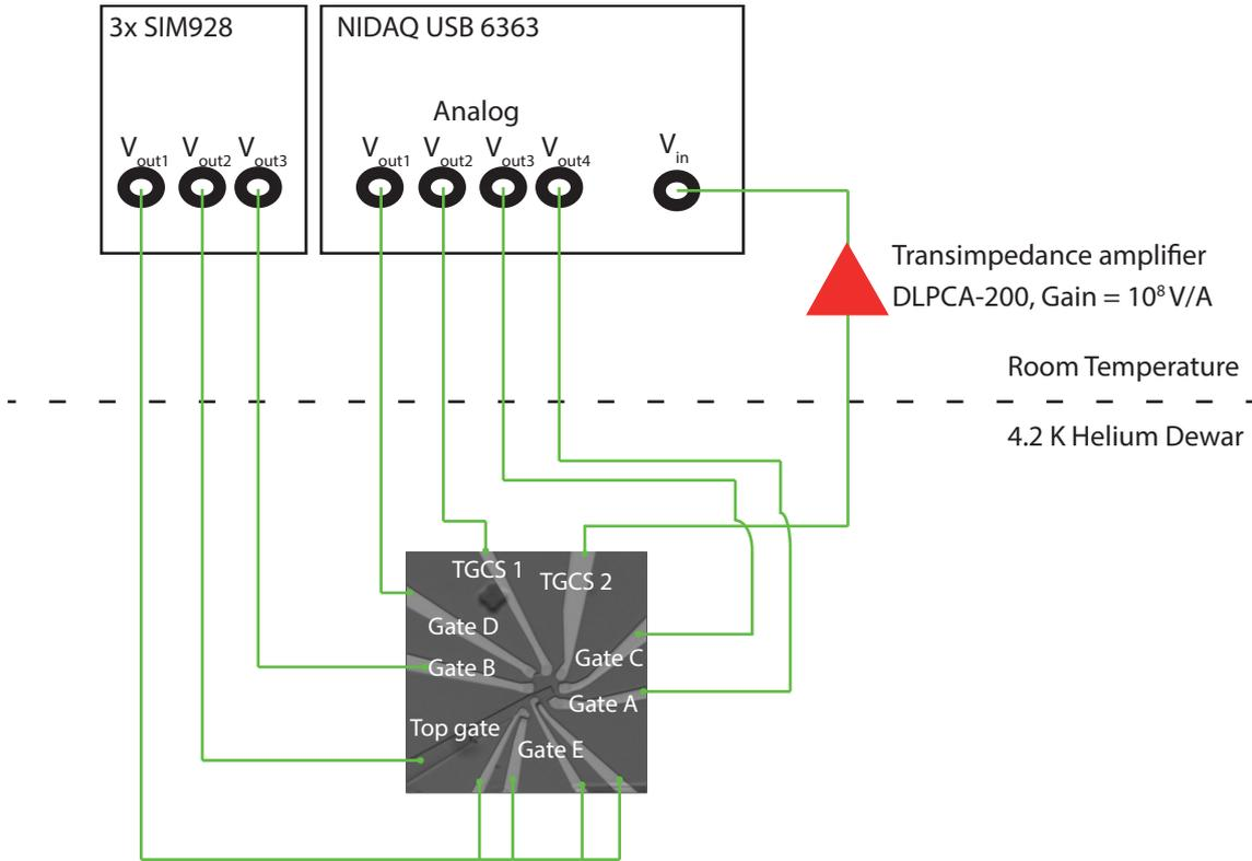
Figure 4.18: Measurement set-up for the 4-dot device primarily consisting of NIDAQ 6363 data acquisition module and SIM928 voltage sources. A Femto DLPCA-200 transimpedance amplifier is used for converting current to voltage and amplifying the TGCS current with a gain of  $10^8$  V/A.
