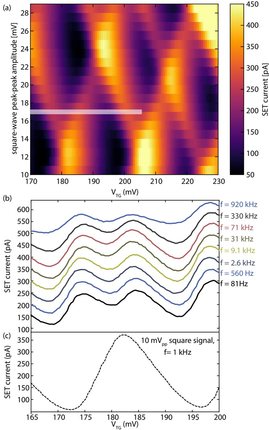
Figure 4.14: Dynamic frequency response of the top gate. (a) Doubling of the coulomb peak is observed after applying a 1 kHz square wave pulse with varying amplitude on the top gate. (b) Frequency response of the square wave pulses up to 920 kHz shown for square wave amplitude of  $17\text{mV}_{pp}$ . (c) A single coulomb peak is shown at  $V_{TG} \sim 180$  mV with a square wave amplitude of  $10\text{mV}_{pp}$  and frequency 1 kHz.
