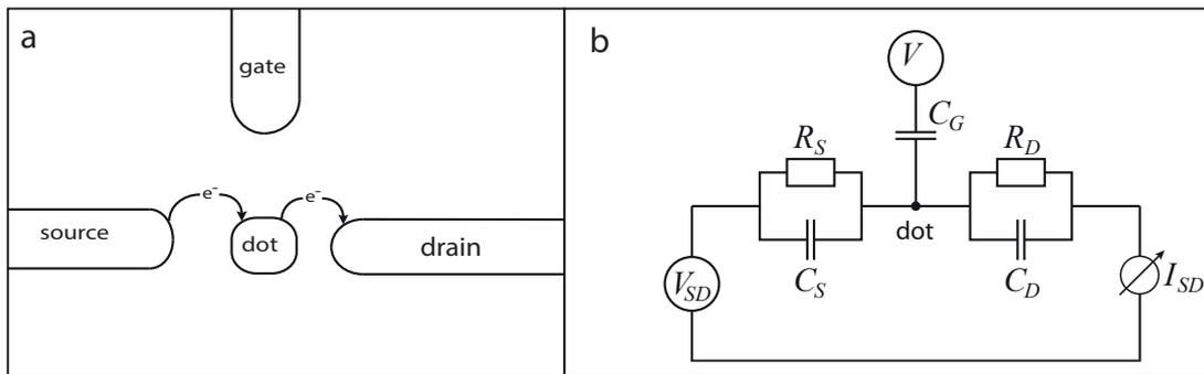
Figure 2.10: Quantum dot device in transport regime. (a) The quantum dot is tunnel coupled to source and drain terminals and capacitively coupled to a gate terminal. (b) A circuit diagram illustrating the quantum dot. Tunnel junctions are modeled as a resistor and capacitor network in parallel. The charging energy of the quantum dot is given by  $e^2/C_{tot}$ , where  $C_{tot}$  is the self capacitance of the quantum dot,  $C_{tot} = C_{source} + C_{drain} + C_{gate}$ .
