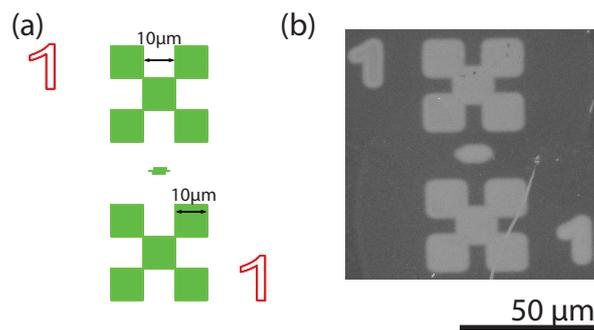
Figure 3.6: Etch Test performed on ALD grown  $\text{Al}_2\text{O}_3$  layers using BHF 1:10 solution maintained at 30 °C. a) Pattern used for etch test defined using EBL. b) SEM image of partially etched  $\text{Al}_2\text{O}_3$  layer obtained after 18 seconds dip in BHF 1:10 solution.
