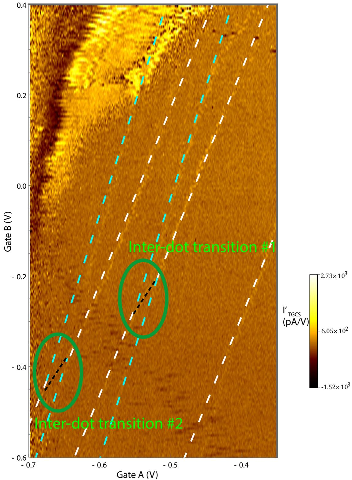
Figure 4.19: Gate-Gate map of the charge transitions from the left hand pair of dots taken by varying gate voltages A and B. Green circles highlight the position of the two inter-dot transitions. Cyan and white color lines have different slopes because they represent the transitions from the bottom and top dots, respectively. The black lines indicate the interdot transitions that were visible when this device was measured in dilution refrigerator.
