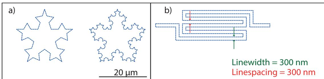
Figure 3.3: Dose test pattern used for  $\text{Al}_2\text{O}_3$  deposited using ALD. a) Koch snowflake fractal pattern used for performing the dose test. b) Finer maze pattern used for dose test. Green arrows give the linewidth and the red arrows indicate the linespacing used in the pattern, with both equaling 300 nm.
