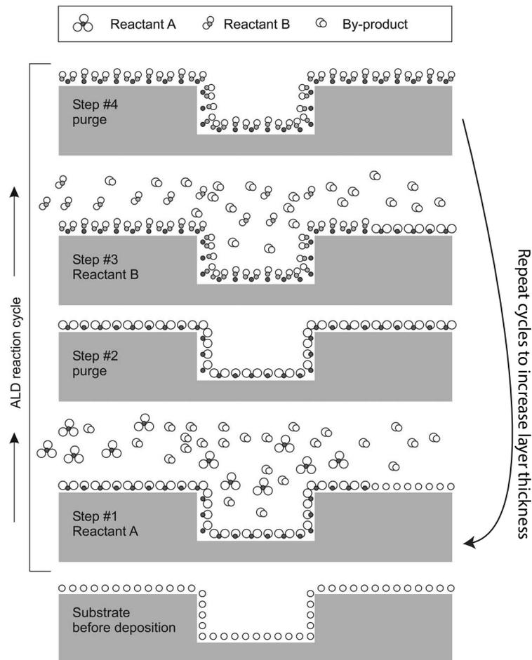
Figure 2.14: Schematic Illustration of one ALD reaction cycle. Figure adapted from [7].
