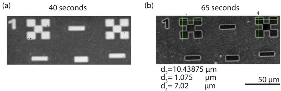
Figure 3.10: Etch test performed on ALD grown  $\text{Al}_2\text{O}_3$  layers using BHF 1:15 solution stored at 20 °C. a) SEM image obtained after 40 seconds dip in BHF 1:15 solution stored at 20 °C showing patterned structures that are not fully etched (as there is no dark contrast). b) SEM image obtained after 65 seconds dip in BHF 1:15 solution stored at 20 °C with fully etched structures giving an average undercut of 1.325  $\mu\text{m}$ .
