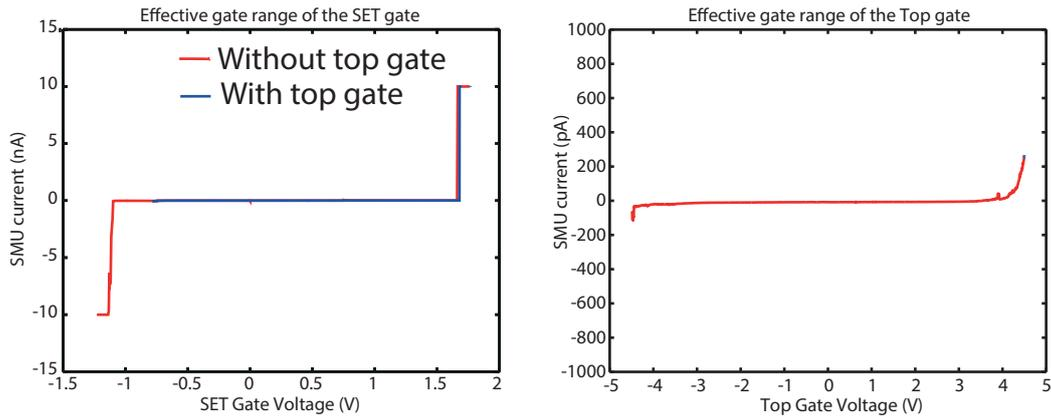
Figure 4.16: Gate leakage curves for the SET gate and the top gate. a) SET gate range before patterning the top gate. b) Effective gate range of top gate.
