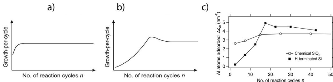
Figure 2.17: a) Dependency of the GPC on the number of reaction cycles showing substrate-inhibited type-1 growth. b) Dependency of the GPC on the number of cycles showing substrate-inhibited type-2 growth. c) Experimental confirmation of substrate-inhibited type-1 and type-2 growth mechanism observed in silicon surface covered with SiO<sub>2</sub> and hydrogen terminated silicon surface, respectively. Figure adapted from [7].
