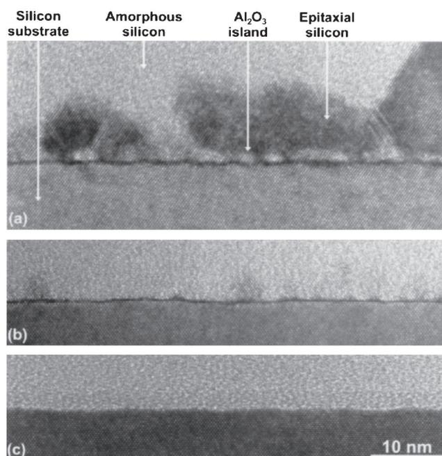
Figure 2.18: Cross-sectional Transmission Electron Microscope image for  $\text{Al}_2\text{O}_3$  deposited on hydrogen terminated silicon at 300 °C showing three cases. a) 15 reaction cycles, b) 20 reaction cycles, and c) 30 reaction cycles. All the grown layers were then capped *in situ* silicon. Figure adapted from [125].
