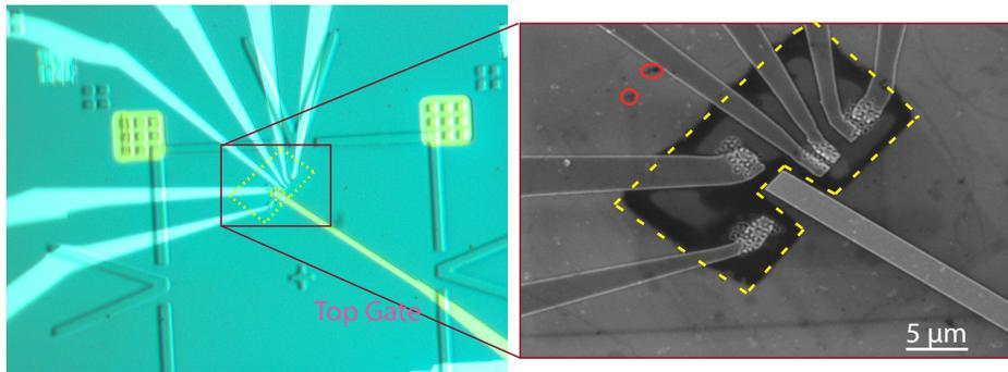
Figure 4.11: Optical (left) and SEM (right) image of the patterned top gate along with the ohmics for the SET quantum dot device. The dashed yellow box in the SEM image on the right is drawn to simply aid in determining the precise placement of the top gate over the the dielectric using the red encircled features as markers.
