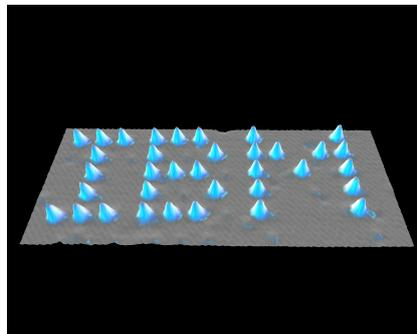
Figure 2.3: 35 Xenon atoms positioned on Ni surface to write IBM, using a STM tip by Eigler in 1990. Figure adapted from [29].
