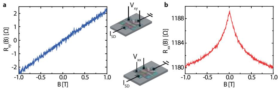
Figure 2.6: Typical magnetotransport measurement of a Si:P  $\delta$ -layer at 4.2 Kelvin with  $n_s \sim 2 \times 10^{14} \text{ cm}^{-2}$ . (a) Hall trace of  $R_{xy}$  used to obtain carrier density, and (b)  $R_{xx}$  used to obtain resistivity and carrier mobility of electrons in a  $\delta$ -layer. Figure adapted from [35].
