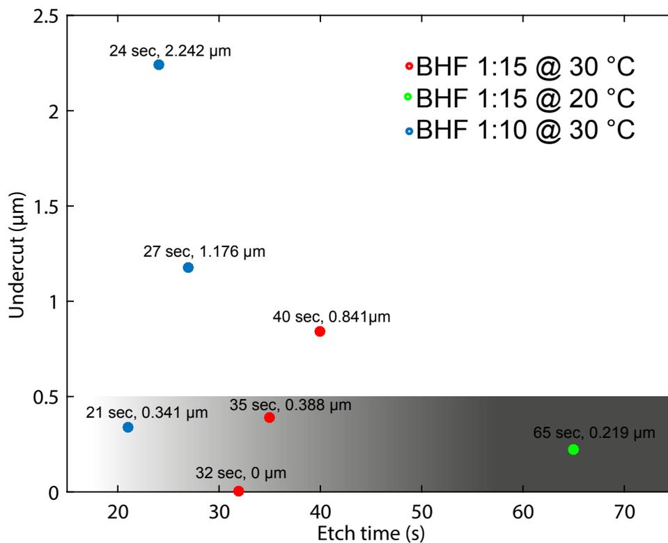
Figure 3.11: Analysis of etching times versus undercut for BHF 1:15 at  $30^\circ\text{C}$ , BHF 1:15 at  $20^\circ\text{C}$  and BHF 1:10 at  $30^\circ\text{C}$ . Shaded region shows the desired area of operation for STM fabricated devices keeping the undercut less than 500 nm.
