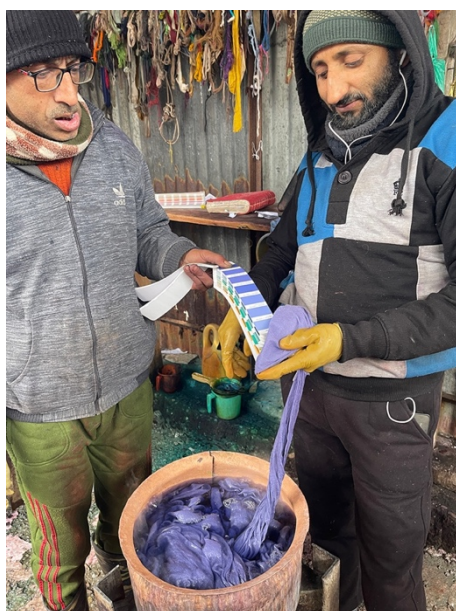
Figure 5.15. Dyer artisan Shabir colour matches synthetically dyed pashmina using a Pantone colour card. Digital photograph by Deborah Emmett.
