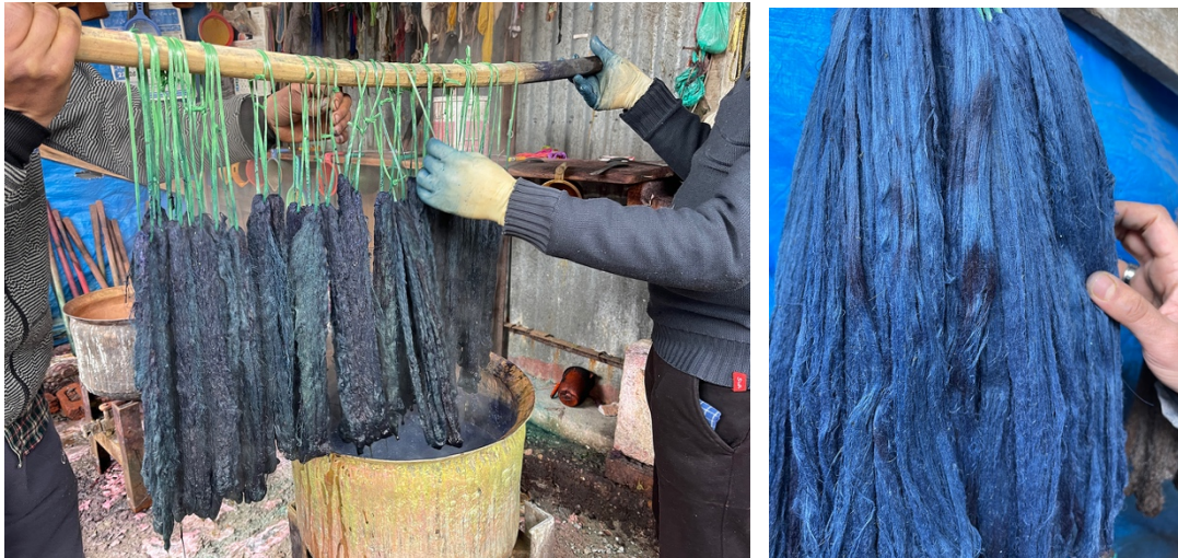
Figure 5.17. Shabir holding the indigo dyed pashmina hanks that are oxidising, turning blue, after removal from the dye vat and the pashmina yarn after drying. Digital photographs by Deborah Emmett.
