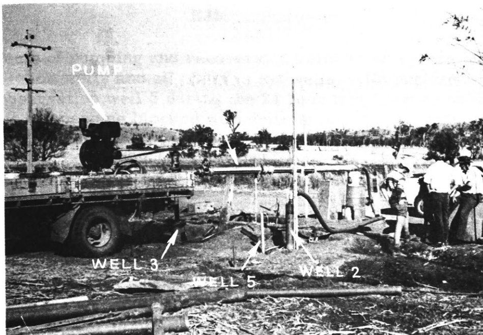
Fig. 3.5: General view of insitu two well testing arrangement.
