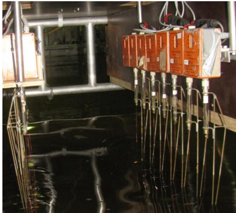
Figure 3.9- Capacitance wave probes used to record water surface elevations.
