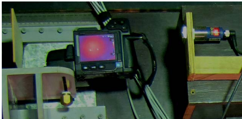
Figure 3.16- The ultrasonic sensor in front of the board connected to the shutter.
