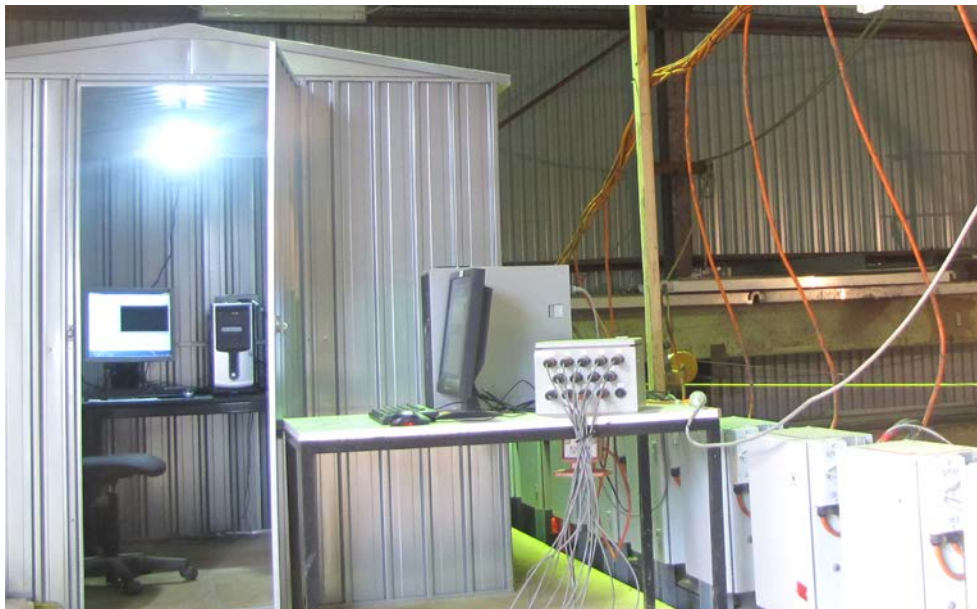
Figure 3.13- The enclosed room to control the TIV system remotely while the laser was operating in the wave basin.
