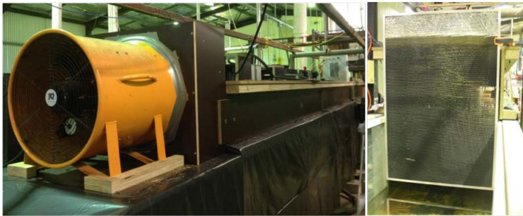
Figure 3.2- The fan and adjustable honeycomb flow guide used to establish a uniform air flow in the 0.6 m flume.
