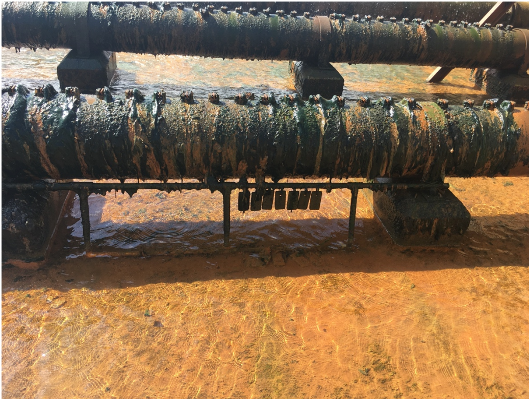
A2.3: Algae growth on the sprinkler pipe and trickling down onto the sprayed vertically placed coupons
