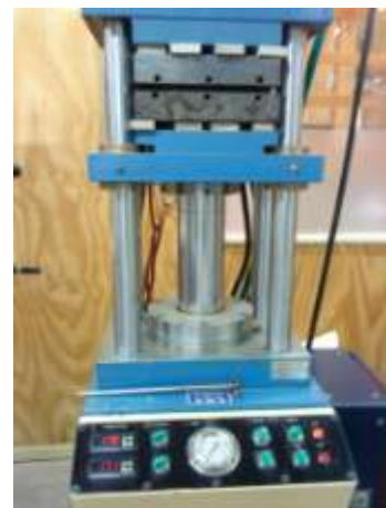
FIGURE 03: Hot platen press with cooling system
