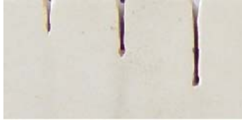
Fig. 1. Kerf characteristics in AWJ multipass cutting with nozzle oscillation (from left to right: single, double and triple pass. u=2\text{mm/s} , P=275\text{MPa} ).
