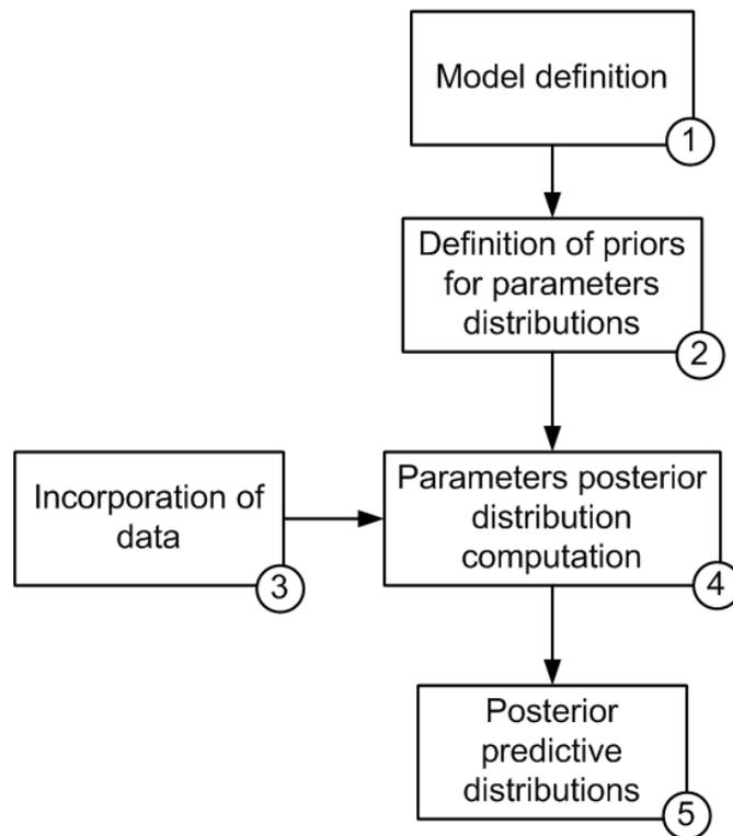
Figure A-7: Construction of posterior and predictive distributions under the Bayesian framework.
