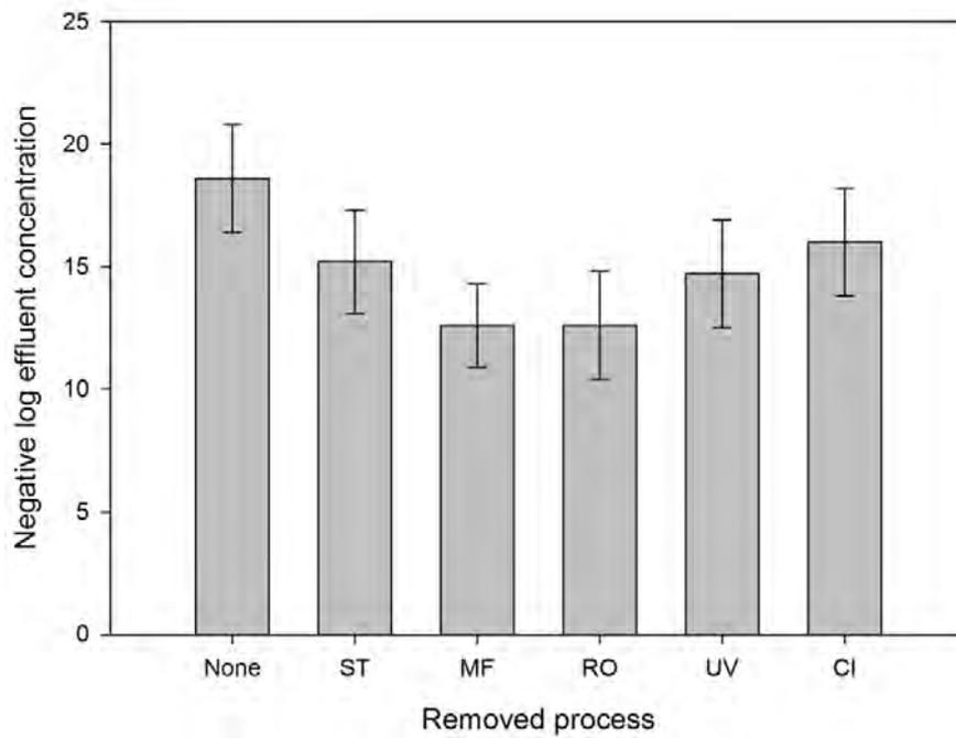
Figure 9-5: Impact of individual process removal for *Salmonella* spp.. ST is secondary treatment; MF is microfiltration; RO is reverse osmosis; UV is UV disinfection, and CL is chlorination. Error bars indicate  $\pm$  standard deviation.
