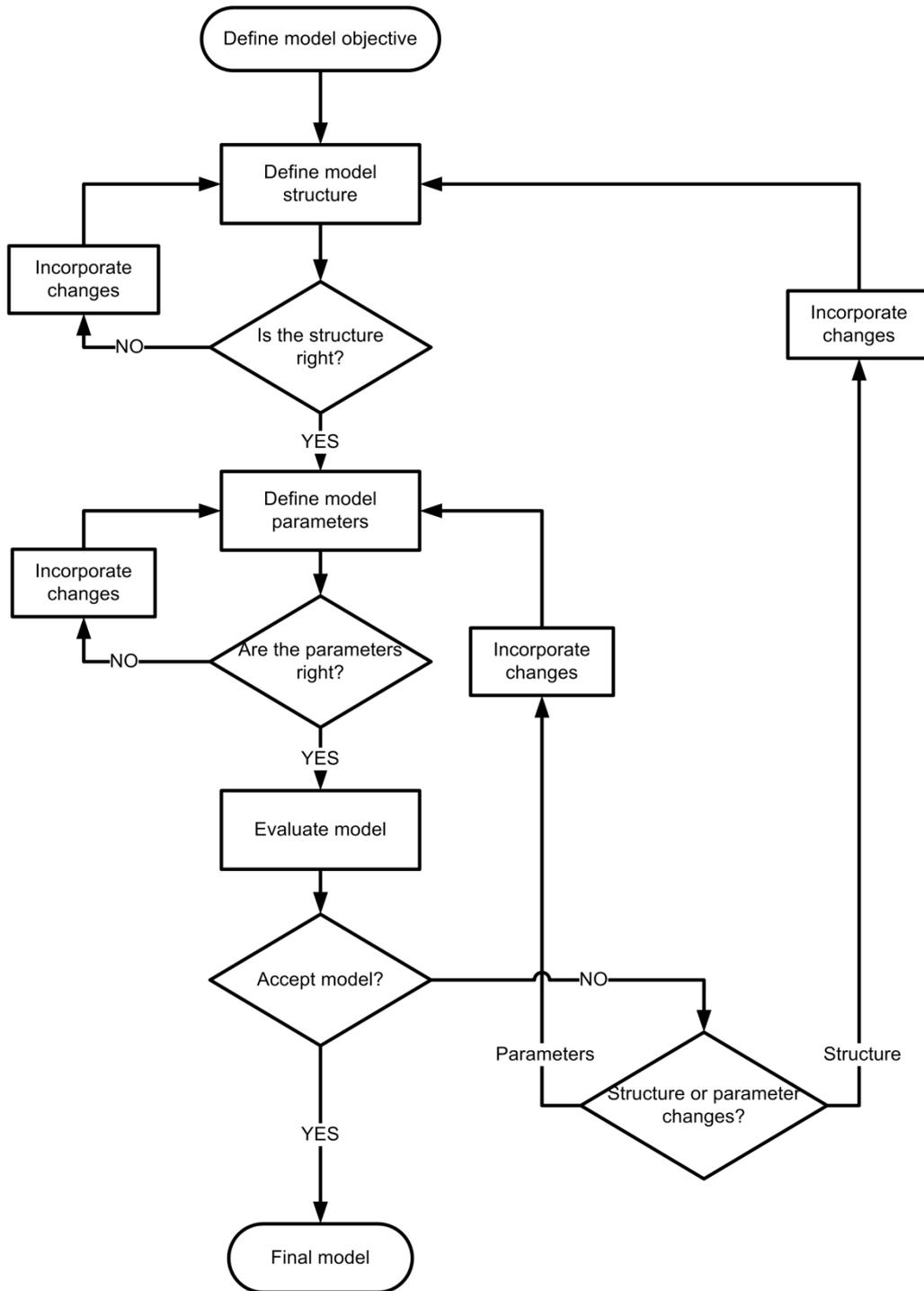
Figure 8-1: Flowchart diagram for BN model development
