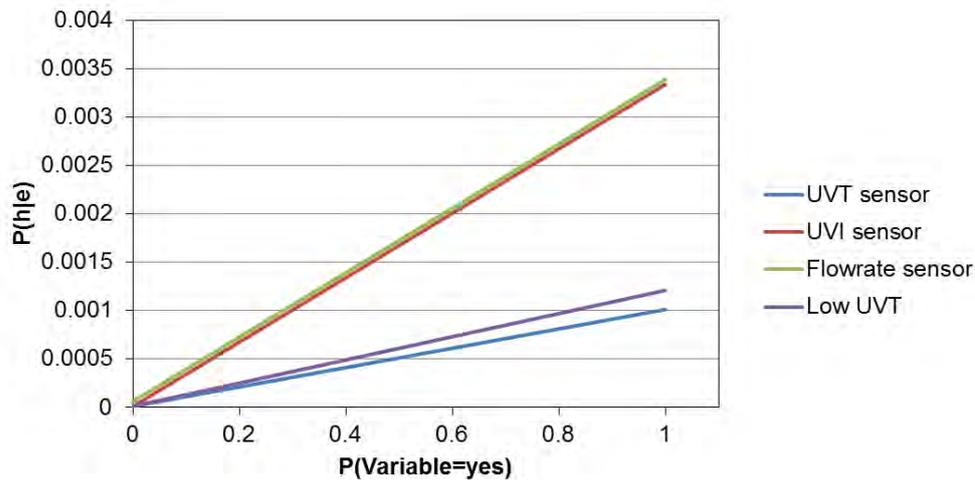
Figure 8-7: Sensitivity of *Low system dose not detected?* to parameters for sensors and *Low UVT*. No evidence was incorporated.
