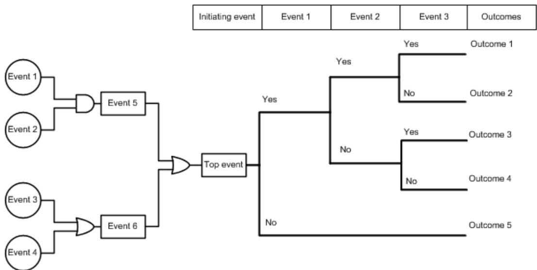
Figure 2-6: Bow-tie representation through FTA and ETA combined
