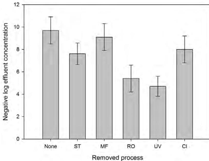
Figure 9-4: Impact of individual process removal for Norovirus. ST is secondary treatment; MF is microfiltration; RO is reverse osmosis; UV is UV disinfection, and Cl is chlorination. Error bars indicate  $\pm$  standard deviation.
