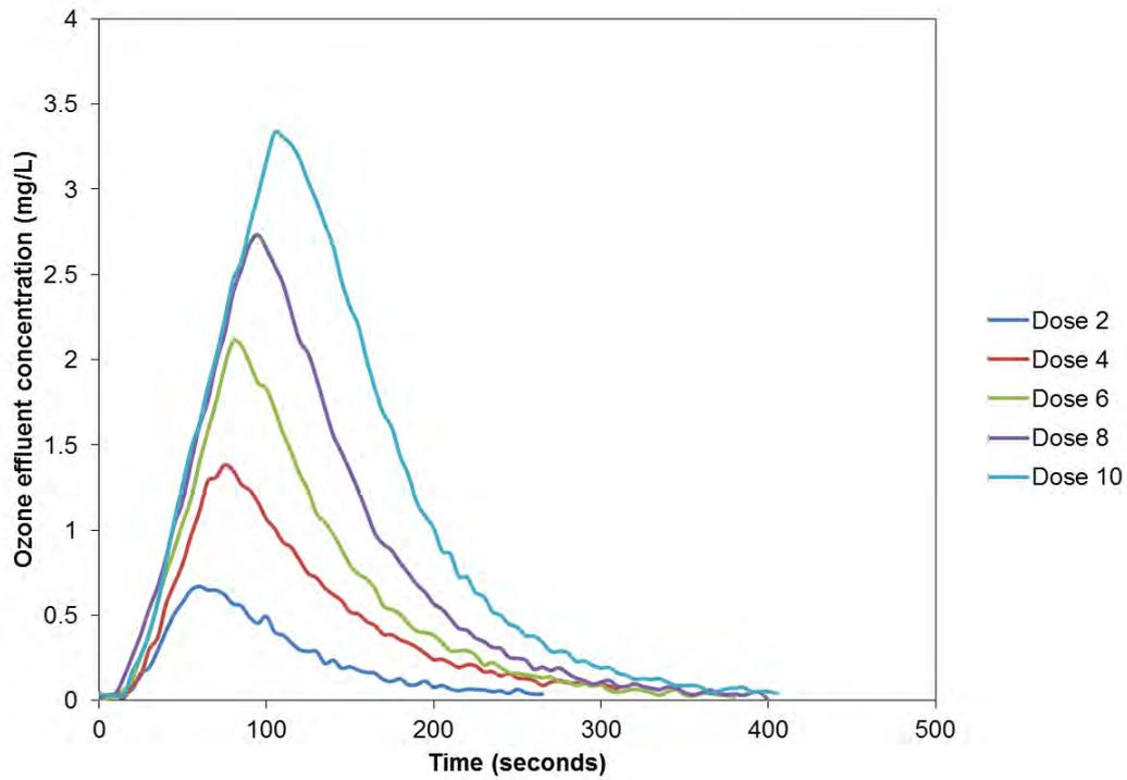
Figure A-15: Average outlet ozone concentration in the gas stream over time
