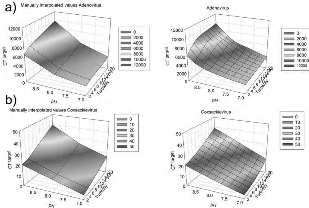
Figure 7-7: Combined effect of pH and turbidity on a) Adenovirus target CT (for LRV 3 ) and b) Coxsackievirus target CT (for LRV 3).
