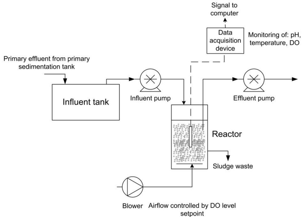
Figure 4-2: Scheme of the activated sludge reactor
