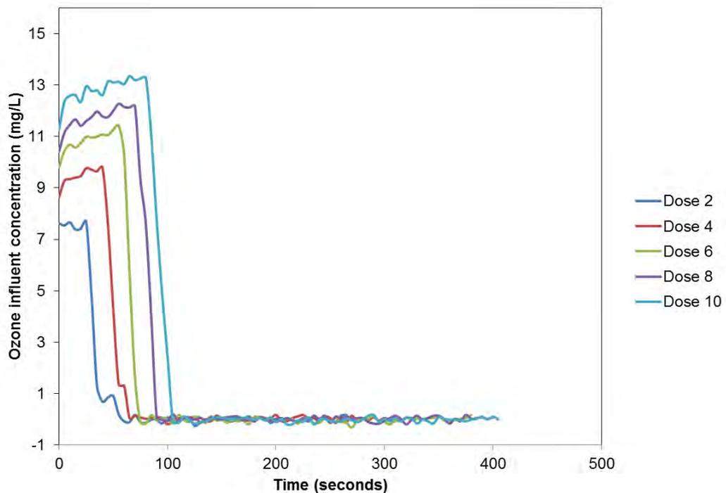
Figure A-14: Average inlet ozone concentration in the gas stream over time
