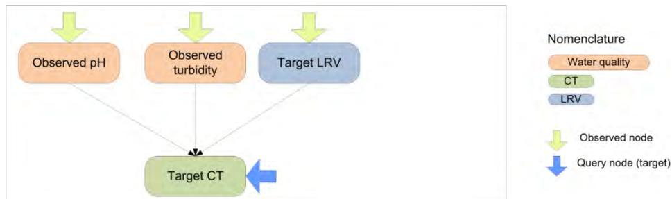
Figure A-19: Scheme of query for target CT given observations of pH, turbidity and LRV.
