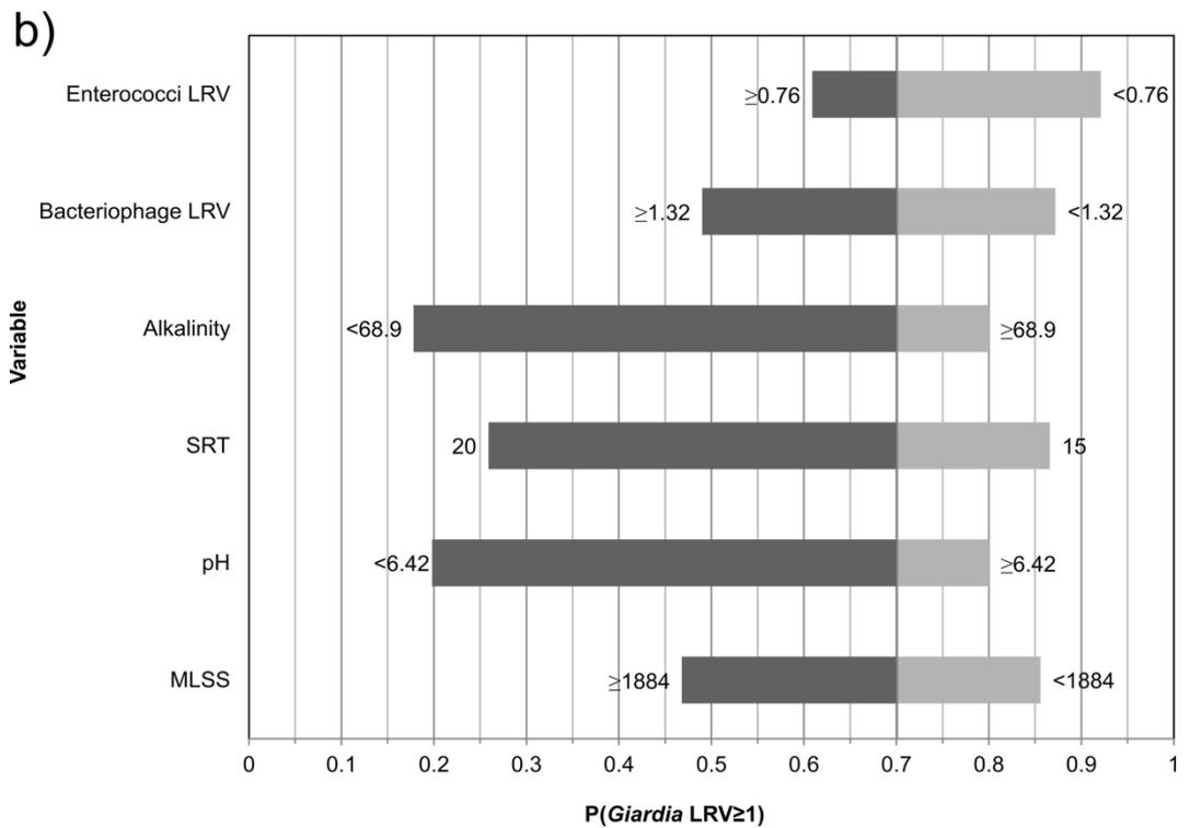
Figure A-4: Sensitivity to findings for removal efficiencies according to most important operating parameters for *C. parvum* BAN model (a) and *G. lamblia* BAN model (b). Bar lengths represent the change in the probability of the state LRV≥1.
