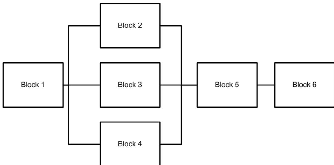
Figure 2-4: Reliability block diagram representation.
