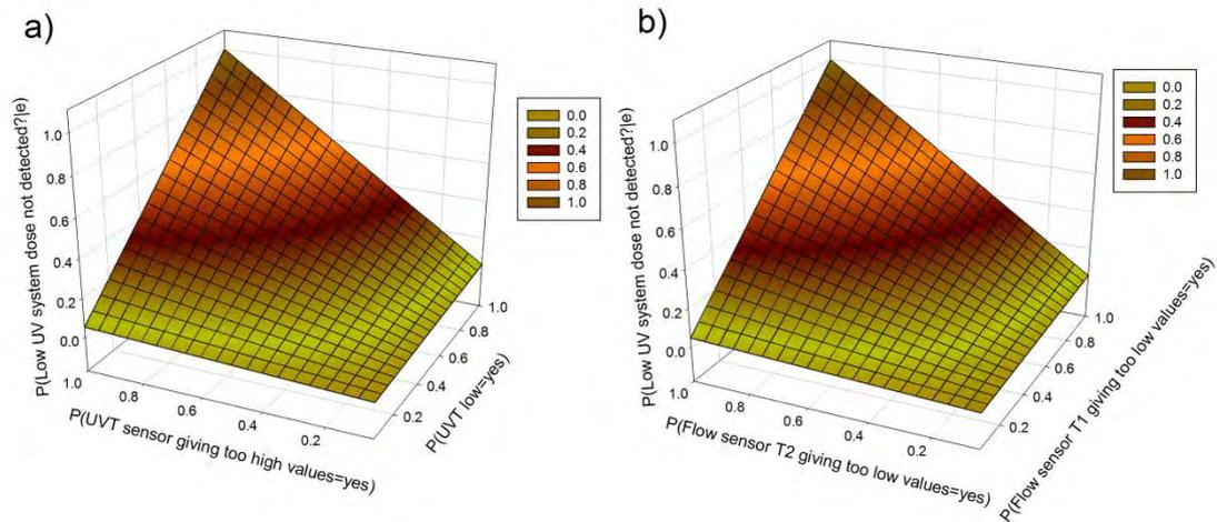
Figure 8-8: Sensitivity of *Low system dose not detected?* to pair of parameters a) UVT low and UVT sensor giving too high values and b) Flow sensors T1 and T2 giving too low values. No evidence was incorporated.
