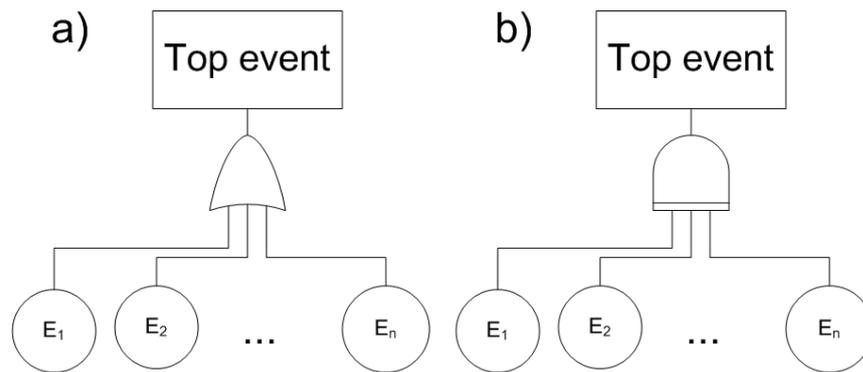
Figure 8-2: Representation of gates of FTA used in this study. a) OR gate, b) AND gate.
