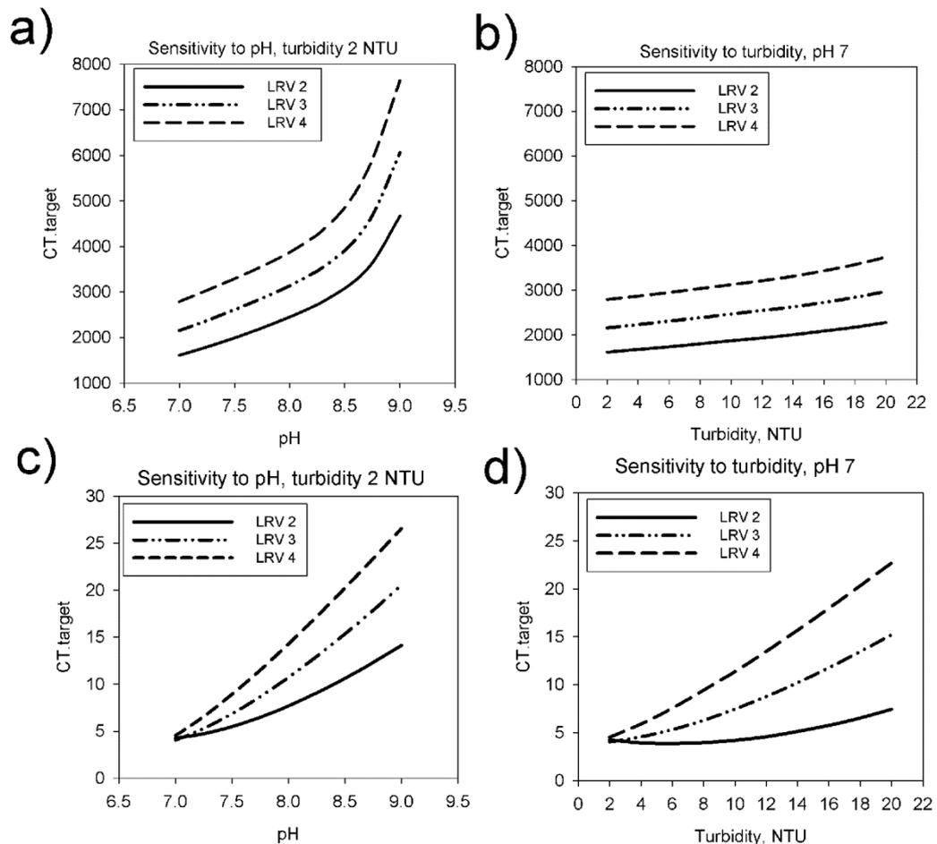
Figure 7-6: Sensitivity of target CT to turbidity and pH for LRV 2, 3 and 4. Sensitivity to, a) pH for Adenovirus and chloramination, b) turbidity for Adenovirus, c) pH for Coxsackievirus and chlorination and d) turbidity for Coxsackievirus.
