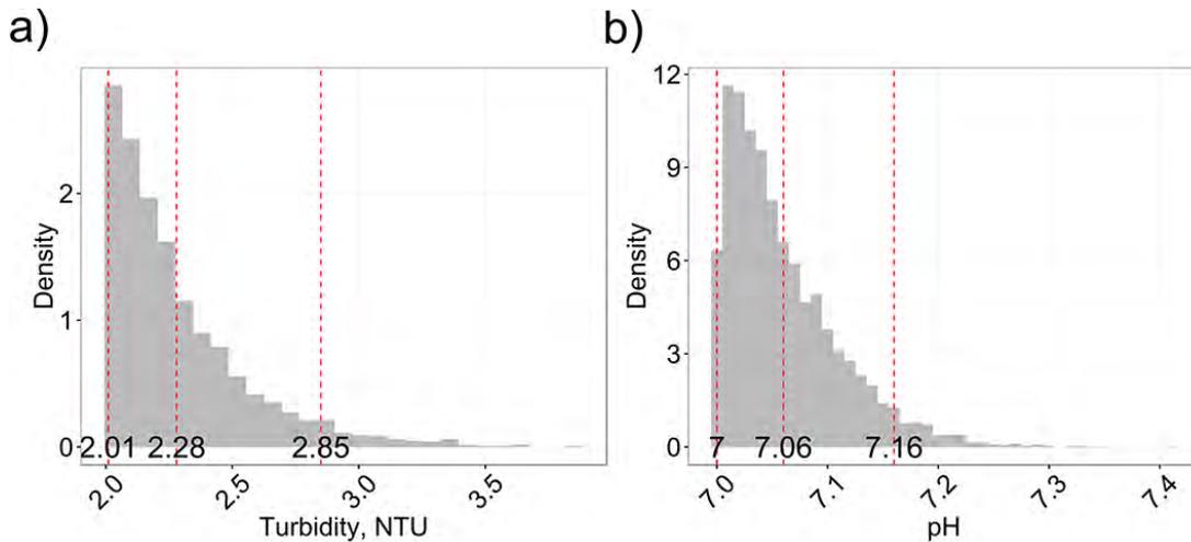
Figure 7-5: Posterior distribution for turbidity and pH after observing CT=20 mg.L<sup>-1</sup>.min and LRV 4 with pH=9 (a) and turbidity 20 NTU (b) for free chlorine.
