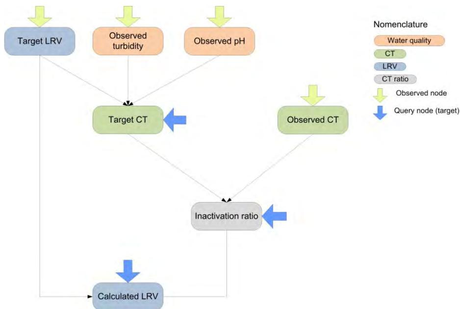
Figure A-21: Scheme of query for inactivation ratio and calculated LRV when the CT is exceeding the range of the study. The required observations are pH, turbidity, target LRV and observed CT.
