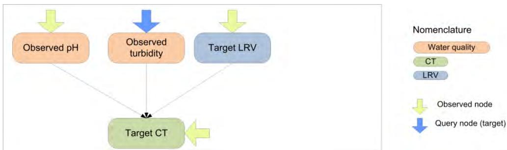
Figure A-20: Scheme of query for required turbidity given observations of pH, required LRV and observed CT.
