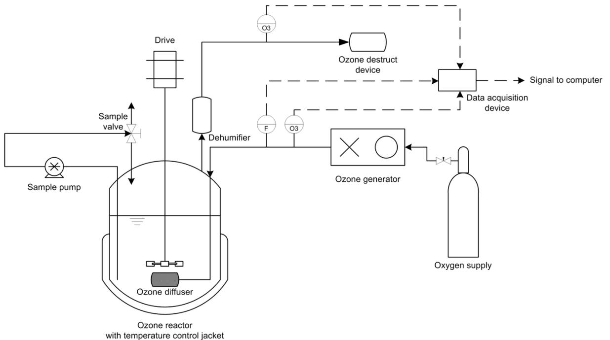
Figure 6-1: Process diagram of the bench-scale ozonation system
