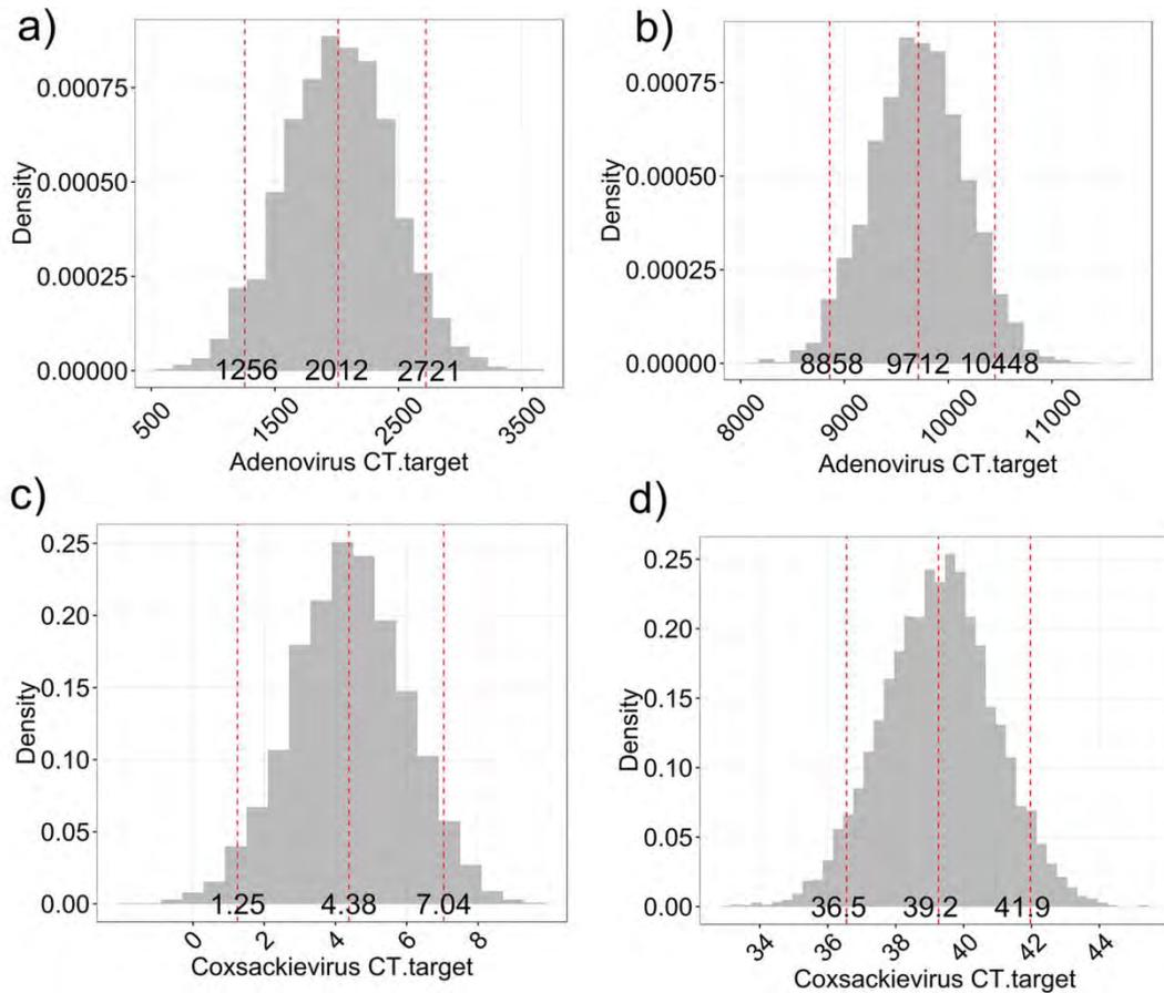
Figure 7-8: CT posterior probability distribution for optimum and worst conditions of pH and turbidity with a LRV of 3. Panels indicate Adenovirus under a) optimum (pH=7, turbidity=2), and b) worst (pH=9, turbidity=20) conditions, and Coxsackievirus under c) optimum (pH=7, turbidity=2), and d) worst (pH=9, turbidity=20) conditions.
