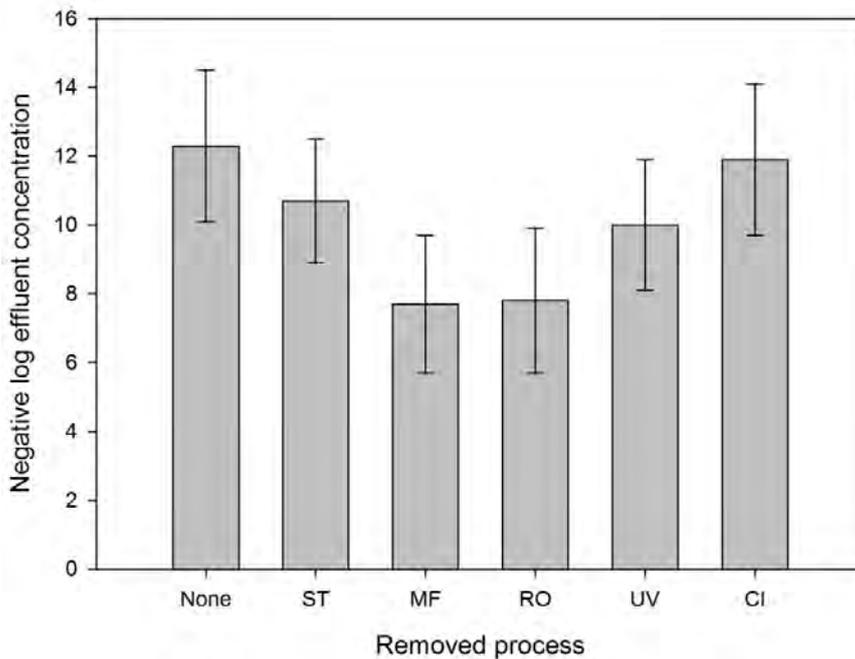
Figure 9-6: Impact of individual process removal for *Cryptosporidium spp.*. ST is secondary treatment; MF is microfiltration; RO is reverse osmosis; UV is UV disinfection, and CL is chlorination. Error bars indicate  $\pm$ standard deviation.
