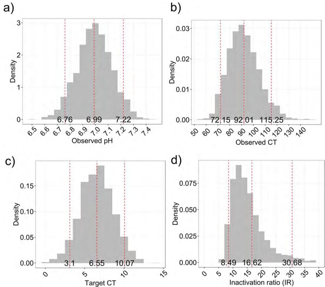
Figure 7-4: LRV estimation using, a) observed pH and, b) CT distributions during a real chlorination process (Walker *et al.*, 2016). The target CT c) is obtained from the BMLP model and the inactivation ratio d) is the ratio between the observed CT and target CT.
