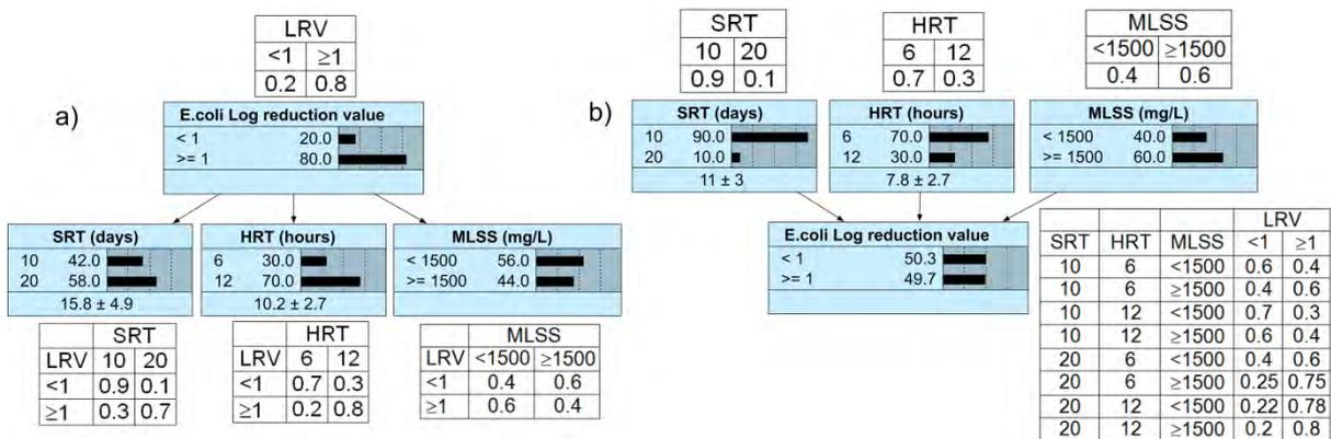
Figure A-1: Non-causal a) and causal Bayesian networks b). Nodes indicate variables and bars indicate the frequencies of each state. Conditional and marginal probabilities are shown in tables.
