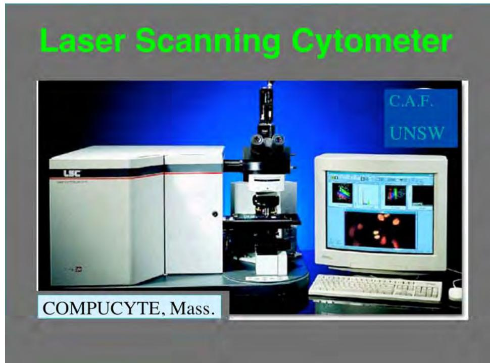
**Figure 2-2 Laser Scanning Cytometer**
