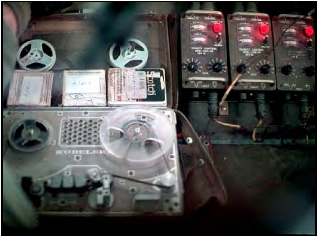
Photograph 21 : Photograph showing a commercial model Kudelski five inch reel-to-reel tape recorder broadcasting from inside a 161 Reconnaissance Flight Pilatus Porter aircraft in Phuoc Tuy province. c. 1971. 214
