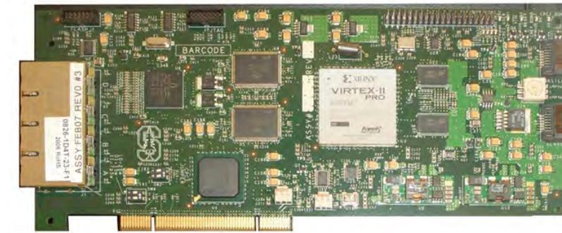
Figure 3.1: An vertical view of the NetFPGA board [4]
