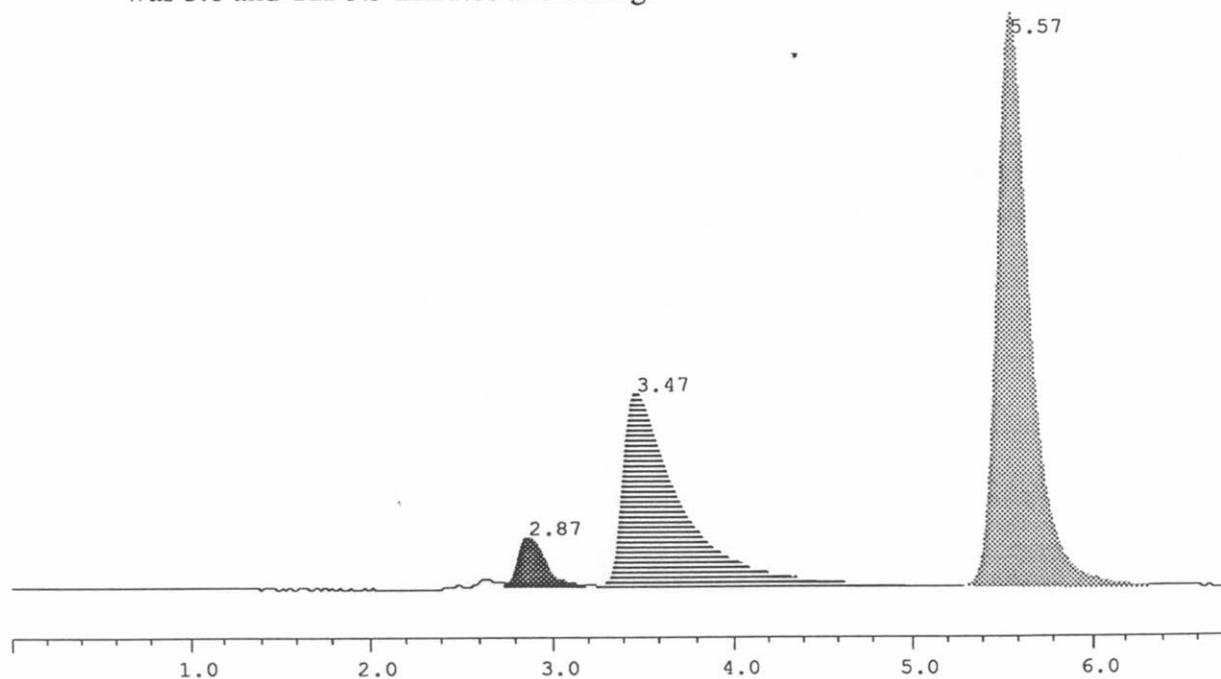
**Fig. 57.** Chromatogram of **TH** and **TQ** standards on the cyano column with hexane/isopropanol (98:2)(solvent system C) as the mobile phase (measured at 280 nm). RT of **TQ** was 2.1 and **TH** 2.4 minutes.
