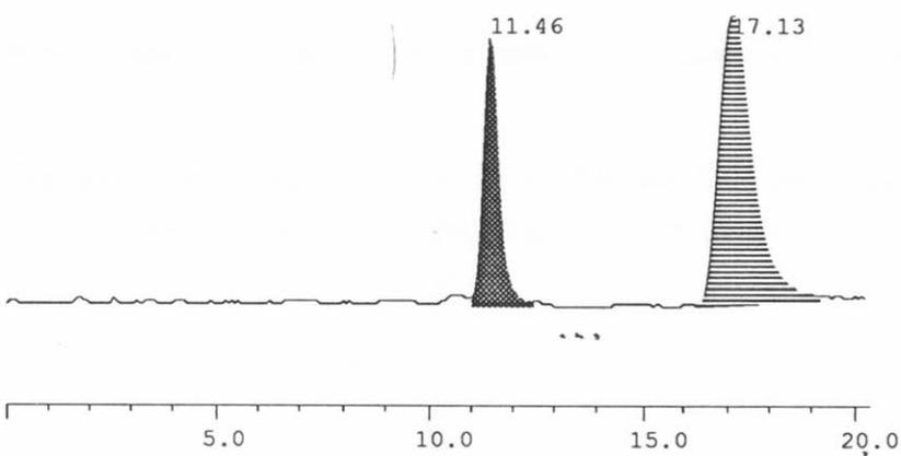
**Fig. 62.** Chromatogram of TOH analysed by RPLC (with methanol/milliQ water (98:2)(solvent J).(RT of TQ was shifted to 13.4 min)
