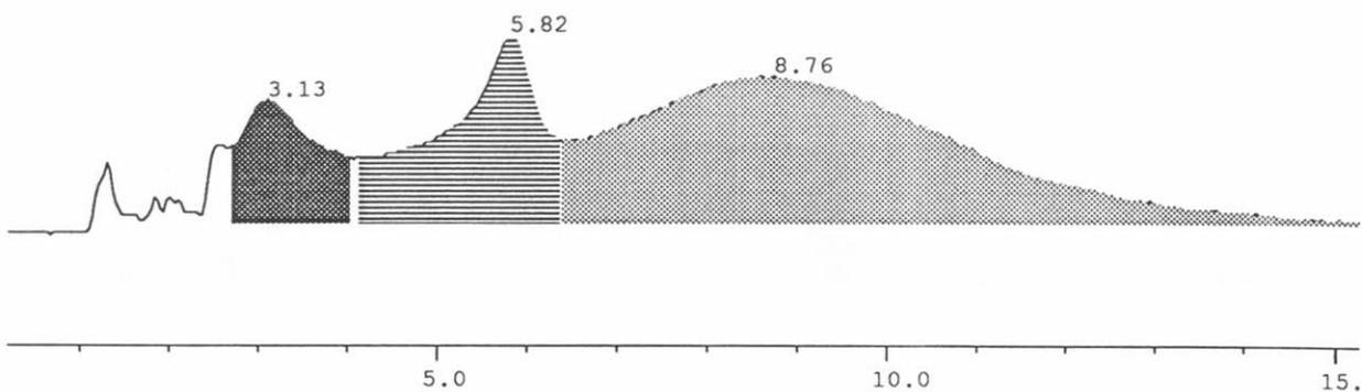
**Fig. 61.** Chromatogram of standard TH and TQ analysed by RPLC (with methanol/milliQ water (98:2)(solvent J).(RT of TH was 17.1 min and TQ 11.5 min.
