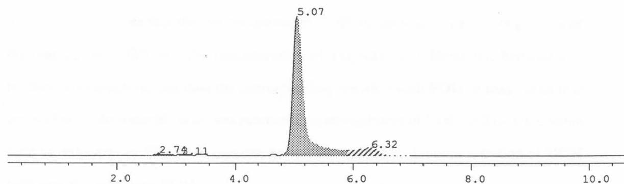
**Fig. 66.** Chromatogram of the reaction between **TOH** and ascorbic acid (10%) for 25 minutes (RT of **TH** was 3.7 and **TQ** 4.9 minutes).
