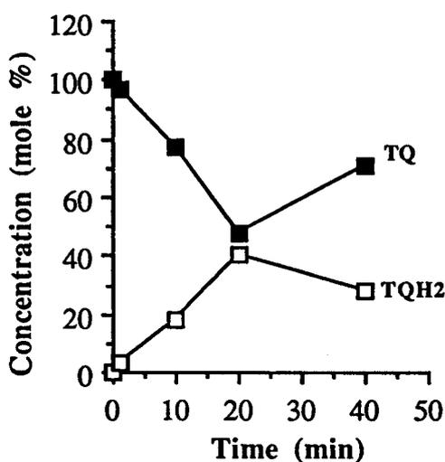
It appeared that reduction of TOH is better with sodium dithionite than with ascorbic acid (at the same concentration), because it reached maximum TH
