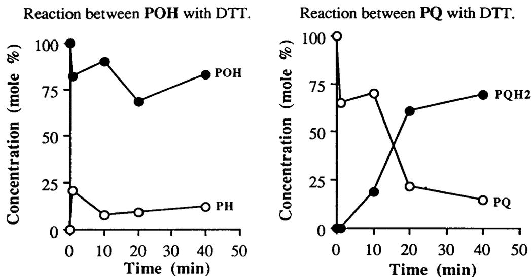
Fig. 47 compares the reactions of POH and PQ with DTT. DTT brings about a small (about 20%) reduction of POH to PH which occurs rapidly and then comes to a halt, while PQH<sub>2</sub> is not formed. By contrast DTT brings about a 70% reduction of PQ to PQH<sub>2</sub> in 40 min and PH is not formed,
