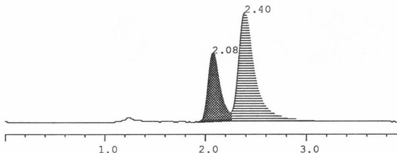
**Fig. 58.** The chromatogram of **TH** and **TQ** standards on the cyano column with hexane/isopropanol (99.25:0.75) as the mobile phase. RT of **TH** was 3.6 and **TQ** 3.9 minutes.
