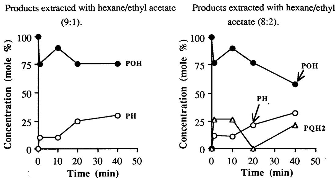
Fig. 51 compares the two extracting solvents on the reaction between **POH** and **DTT**. With the less polar solvent (hexane/ethyl acetate (9:1)), only **PH** is observed as a product, while, with the more polar solvent, some **PQH<sub>2</sub>** was also observed. In this case it appears that the more polar solvent does manage to extract **PQH<sub>2</sub>**.
