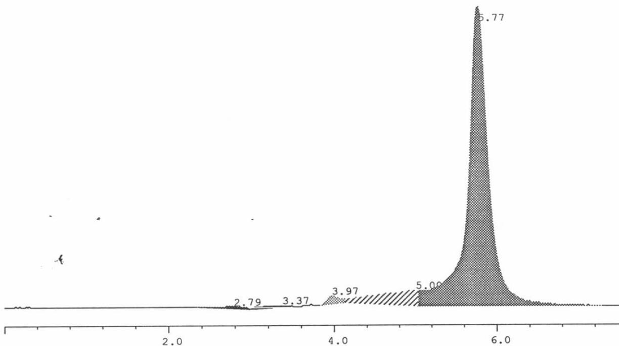
**Fig.56.** Chromatogram of **TH** and **TQ** standards in silica column with hexane/ethyl acetate (4:1)(solvent A) as the mobile phase (measured at 280 nm). RT of **TQ** was 5.6 and **TH** 3.5 minutes and tailing.
