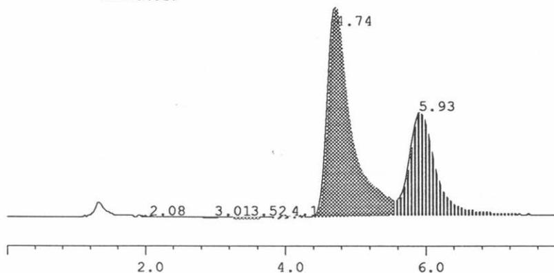
**Fig. 60.** Chromatogram of TQH<sub>2</sub> on the cyano column with hexane-isopropanol (99.5:0.5)
