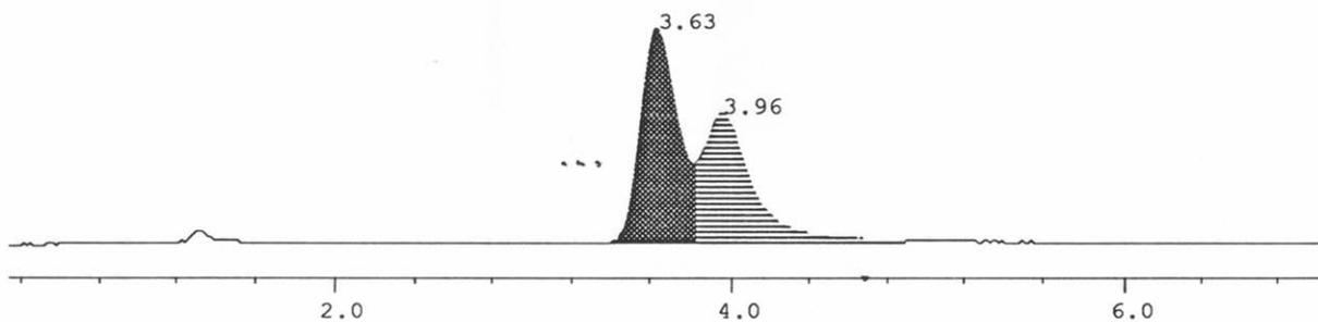
**Fig. 59.** Chromatogram of **TH** and **TQ** standards on the cyano column with hexane-isopropanol (99.5:0.5) as the mobile phase. RT of **TH** was 4.7 and **TQ** 5.9 minutes.
