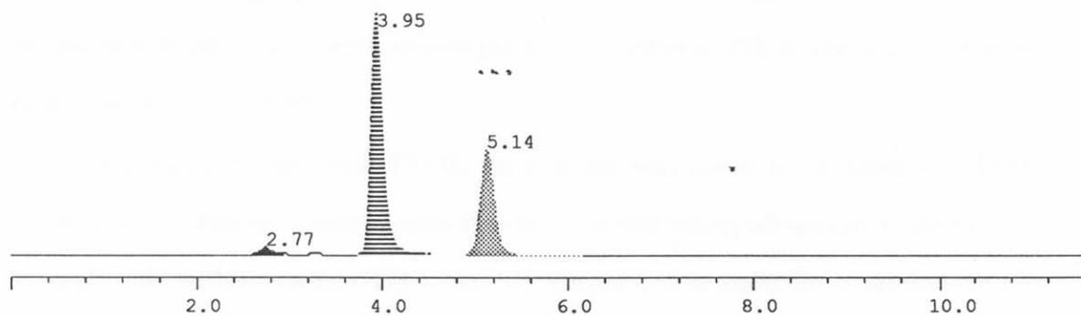
**Fig. 65.** Chromatogram of **TOH** immediately after preparation analysed by NPLC (solvent C: hexane/isopropanol (98:2))(RT of **TQ** was 5.1 min).
