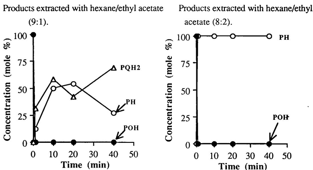
These very different results cannot be explained by the extracting solvent since the more polar solvent hexane/ethyl acetate (8:2) would have been expected to extract more PQH<sub>2</sub>. The reason for the differences may lie in the speed with which sodium dithionite is used after dissolving it in solution. Thus dithionite in solution reacts very rapidly with oxygen, thereby reducing its effective concentration.
