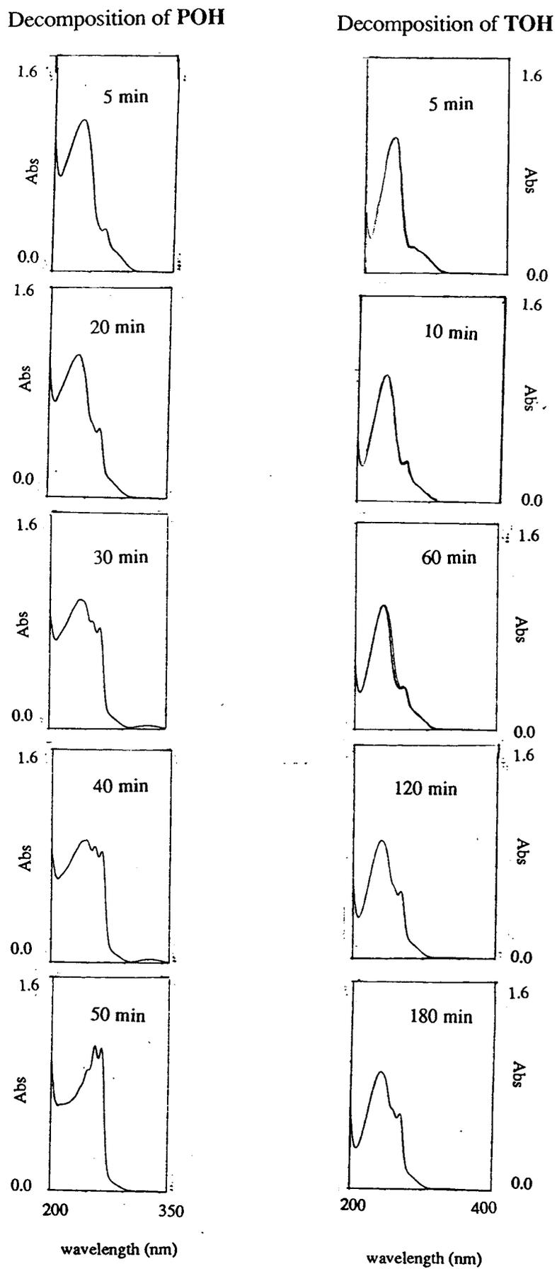
Fig. 54. Rate of decomposition of POH and TOH determined by UV spectrometry.
