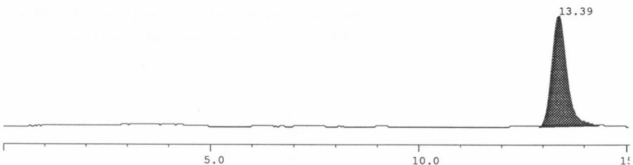
**Fig. 63.** Chromatogram of the reaction between **TOH** and ascorbic acid (10%) for 40 min, analysed by RPLC, solvent (RT of **TQ** is 11.5 min and **TH** 17.1 min).
