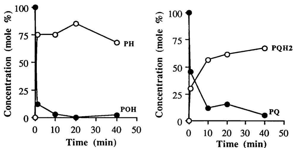
Fig. 46 (p. 182) compares the reactions of **POH** and **PQ** with sodium dithionite, **POH** is almost completely reduced to **PH** within 20 min and no **PQH<sub>2</sub>** formed while **PQ** is reduced more slowly (70% in 40 min) to **PQH<sub>2</sub>** and no **PH** is formed.
