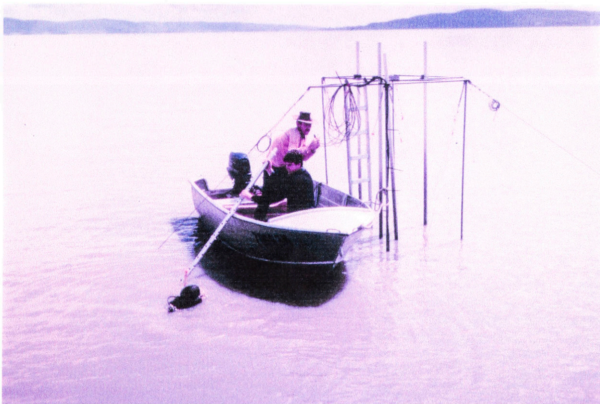
Figure 2.34 Mounting of the Zwarts poles of the directional array after cleaning. Note the diver in the water who is about to install the pole underwater.
