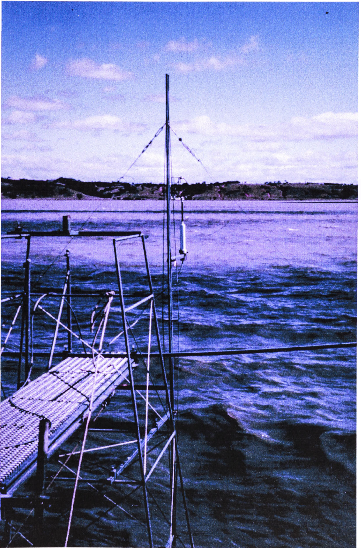
Figure 2.25 A sonic anemometer deployed at the end of the 4m long measurement bridge at the platform (station 6).
