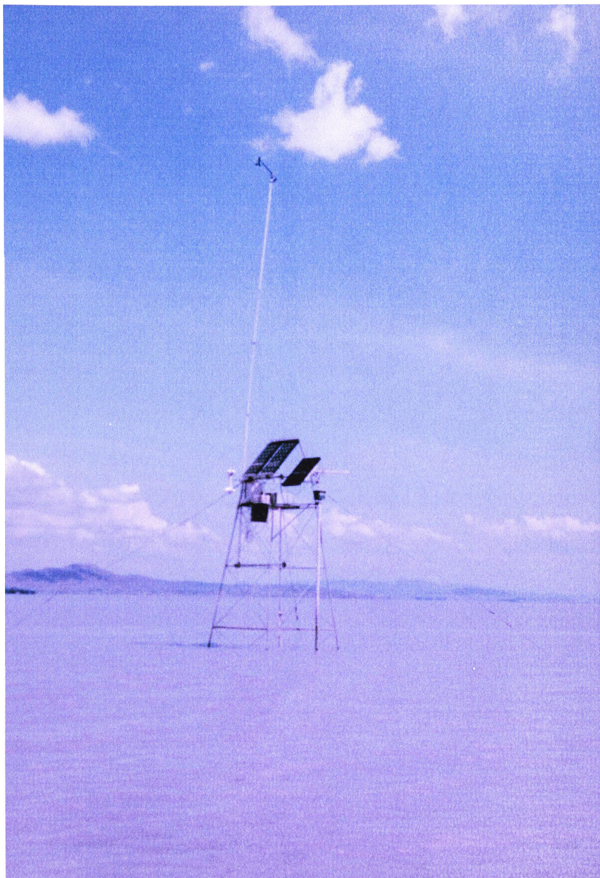
Figure 2.18 Zwarts pole in position on one of the towers. A 10 metre anemometer mast is also placed on this tower. All towers had solar panels that had to be cleared of bird droppings regularly.
