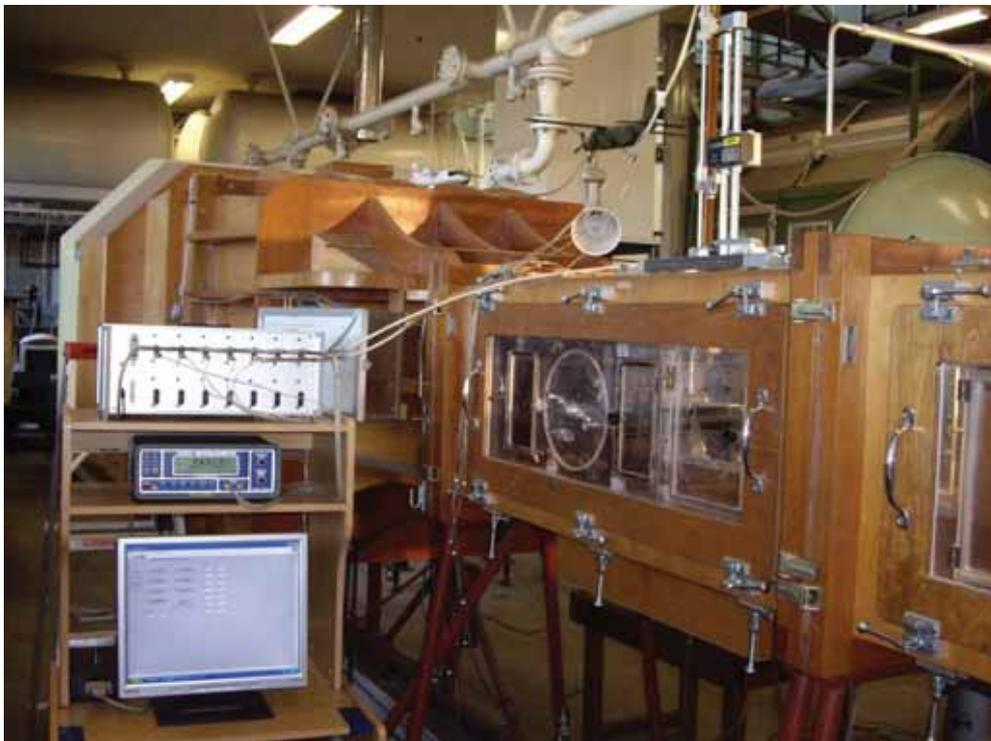
Figure 3.6. Wake traverse apparatus and instrumentation.
