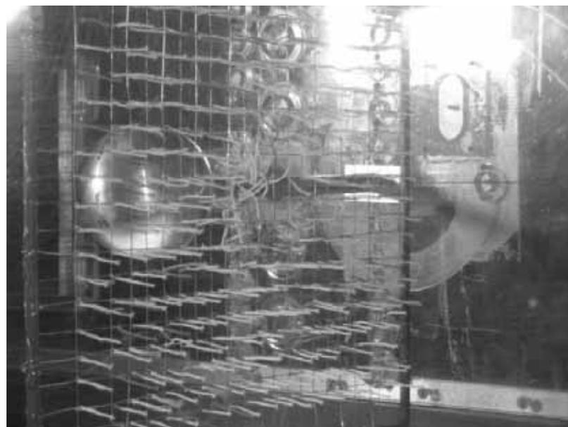
Figure 5.5. Tuft mesh. Flow speed of 10 m/s with synthetic jet. Tuft screen 40 mm offset. A side view of Figure 5.4.
