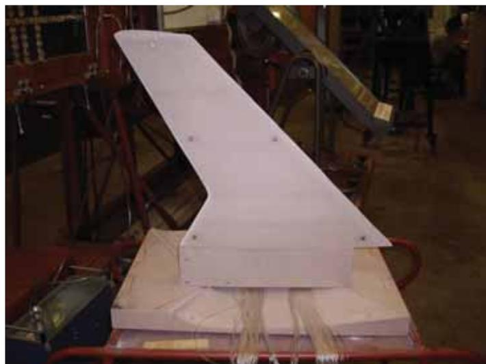
Figure 3.13. Forward swept wing with NACA-23012 profile.
