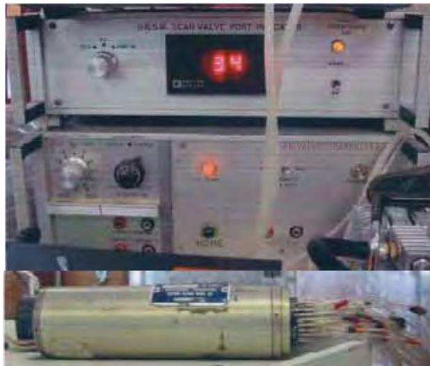
Figure 3.3. Scanivalve controller and scanivalve unit below.
