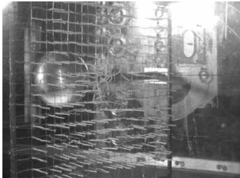
Figure 5.3. Tuft mesh. Flow speed of 10 m/s without synthetic jet. A side view of Figure 5.2
