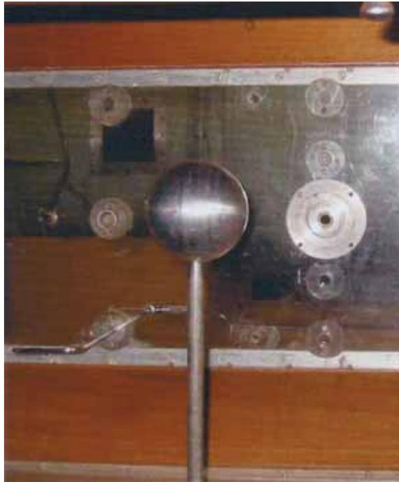
Figure A.3. Side-supported sphere mounted in the 457 mm x 457 mm wind tunnel.
