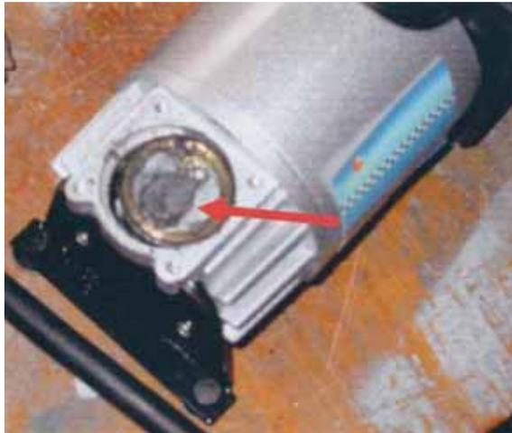
Figure A.7. Compressor one-way valve.
