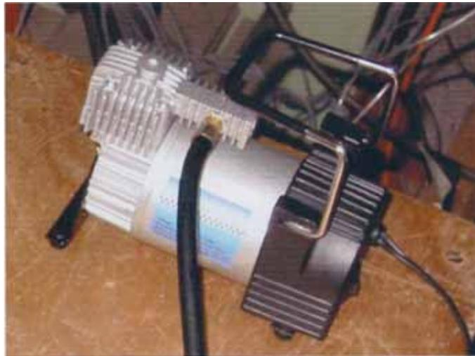
Figure A.6. 12VDC Compressor
