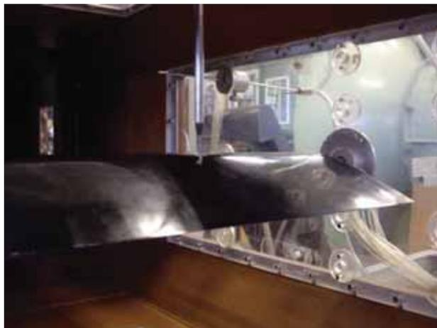
Figure 3.8. five-hole probe wake survey of NACA23012 airfoil
