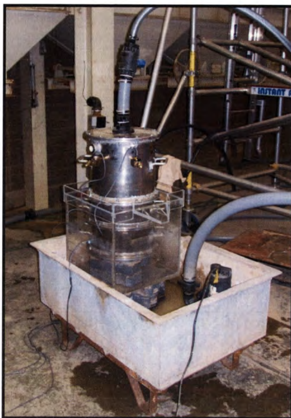
Figure 3.28: Downward flow seepage test apparatus.
