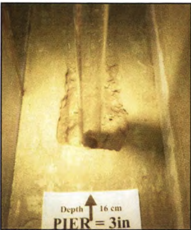
Figure 2.6: Scour hole next to a cylindrical pier in clay during a flume test ( http://tti.tamu.edu/geotech/scour/ ).
