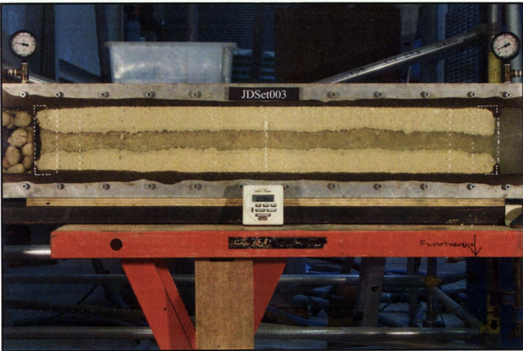
Figure 2.25: Slot Erosion Test on soil sample taken from Jindabyne Dam.
