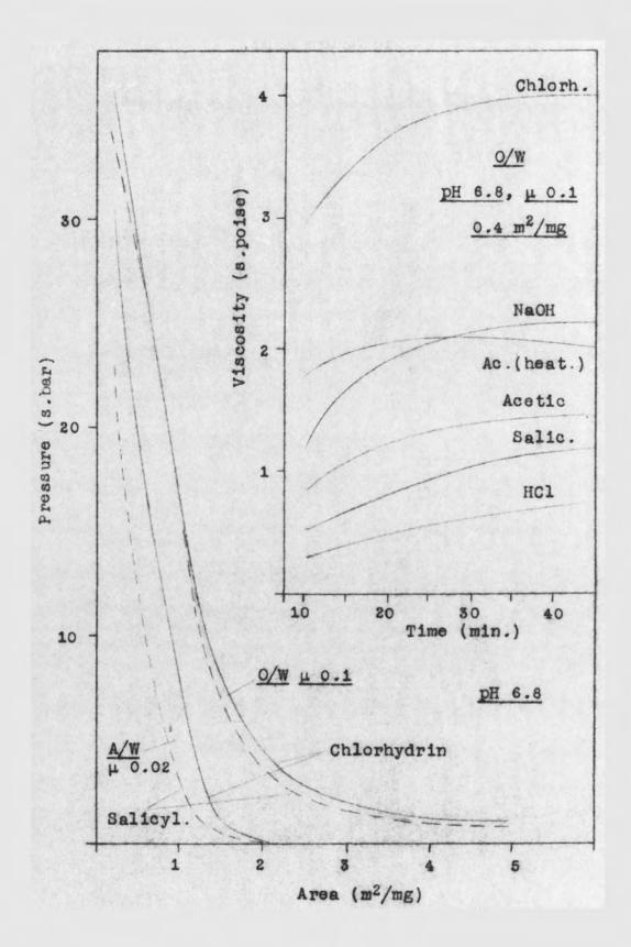
Concentrations of the spreading solution between 0.16 and 0.84 mg/ml were found to have no effect on the isotherms at the O/W interface. Surface pressure measurements at the A/W interface were independent of the initial spreading area within the range 2.0 to 4.0 m<sup>2</sup>/mg. Interfacial viscoelastic measurements at the O/W interface were not influenced by the initial spreading area within the range 1.5 to  $5.0 \text{ m}^2/\text{mg}$ .
