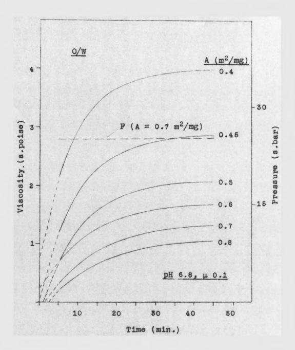
Fig.63b. Interfacial Elasticity-Time Curves (Gluten).
