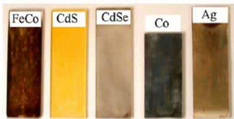
**Figure 2.26** Thin films of FeCo, CdSe, CdS, Co and Ag formed on glass microslides prepared under solvothermal conditions.<sup>[98]</sup>
